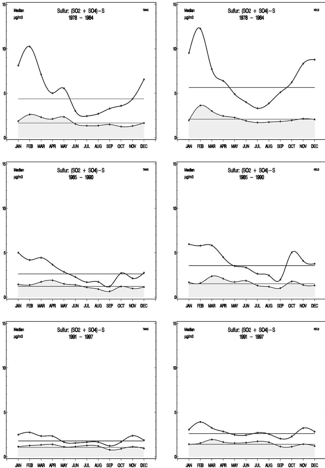
Figure 2.4.1 Average annual behaviour of the sum of monthly median concentrations of sulphur compounds in 3 subperiods. Particulate phases are shaded. Results from station Tange at left and from Keldsnoor at right. The component medians of each subperiod are shown as horizontal lines.
