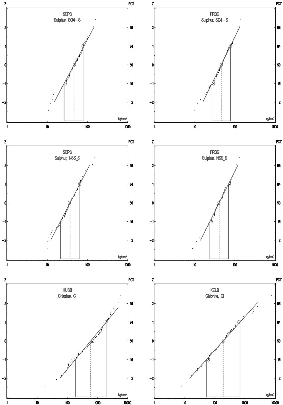
Figure 4.1.3 Statistical distributions of monthly bulk depositions since 1991 of sulphur compounds and chlorine. The depositions are shown logarithmically on the horizontal axis and circles denote the 16-, 50-, and 84-percentiles. The straight line is the log-normal fit through the indicated geometric mean and standard deviations.
