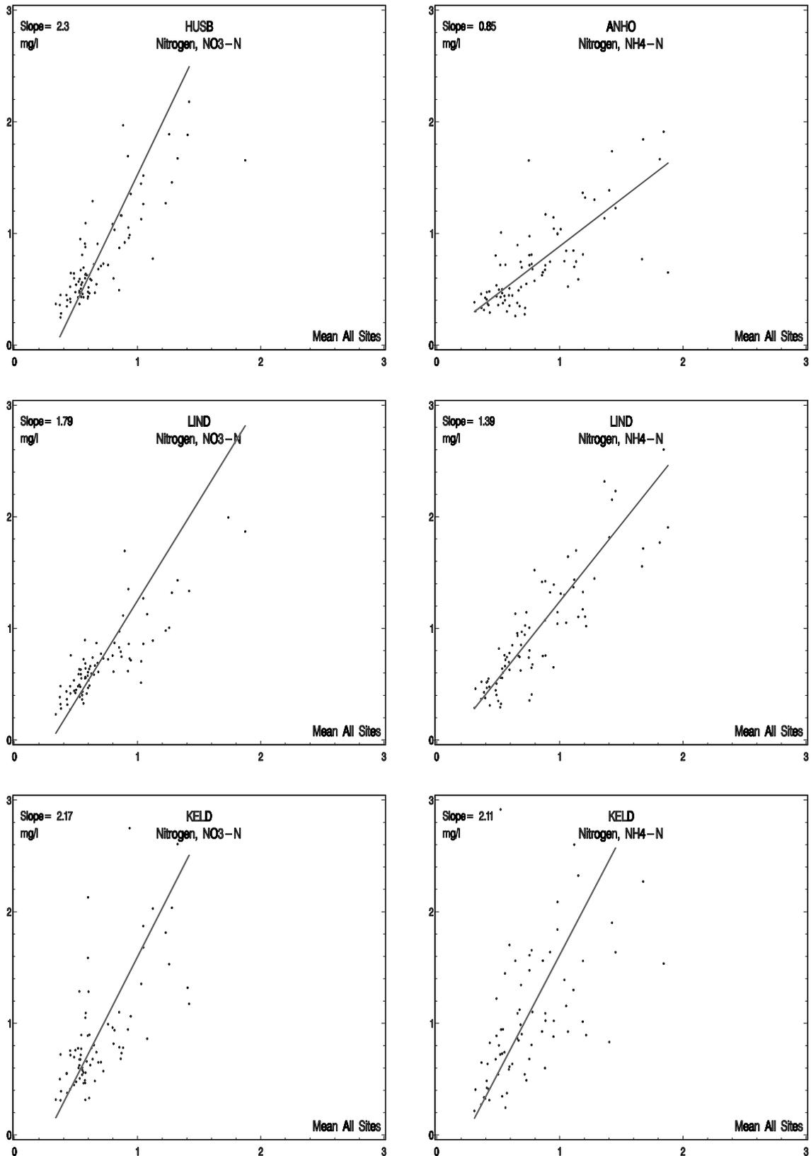
Figure 3.2.2 Monthly precipitation weighted bulk concentrations of nitrogen compounds 1991-1997. Site concentrations plotted and regressed orthogonally against the means at all sites. Calculations are based on all data, whereas displayed data amount to minimum 95% of all.
