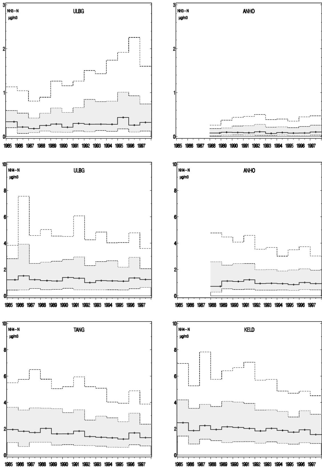
Figure 2.3.2 Annual medians, upper and lower quartiles (shaded) and the 90-percentile of 24h air concentrations reduced nitrogen compounds, gaseous  $\text{NH}_3\text{-N}$  and particulate  $\text{NH}_4^+\text{-N}$  since 1985.
