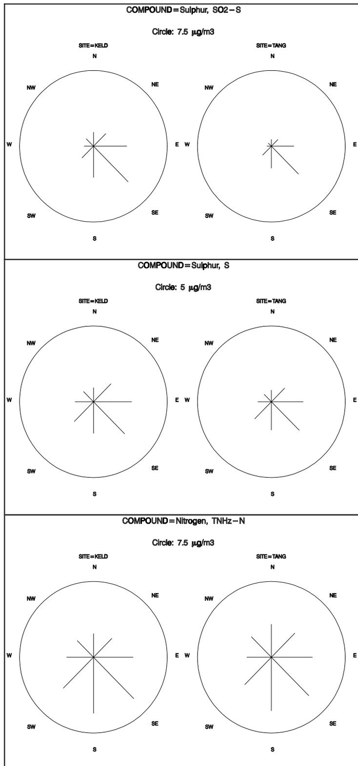
Figure 5.1.1 Mean concentrations of SO<sub>2</sub>, S and TNHz at Keldsnoor and Tange for 1991 – 1997. The sector value is the mean concentration in winds from that direction. For each compound the scale is given by the radius of the circumscribing circle.
