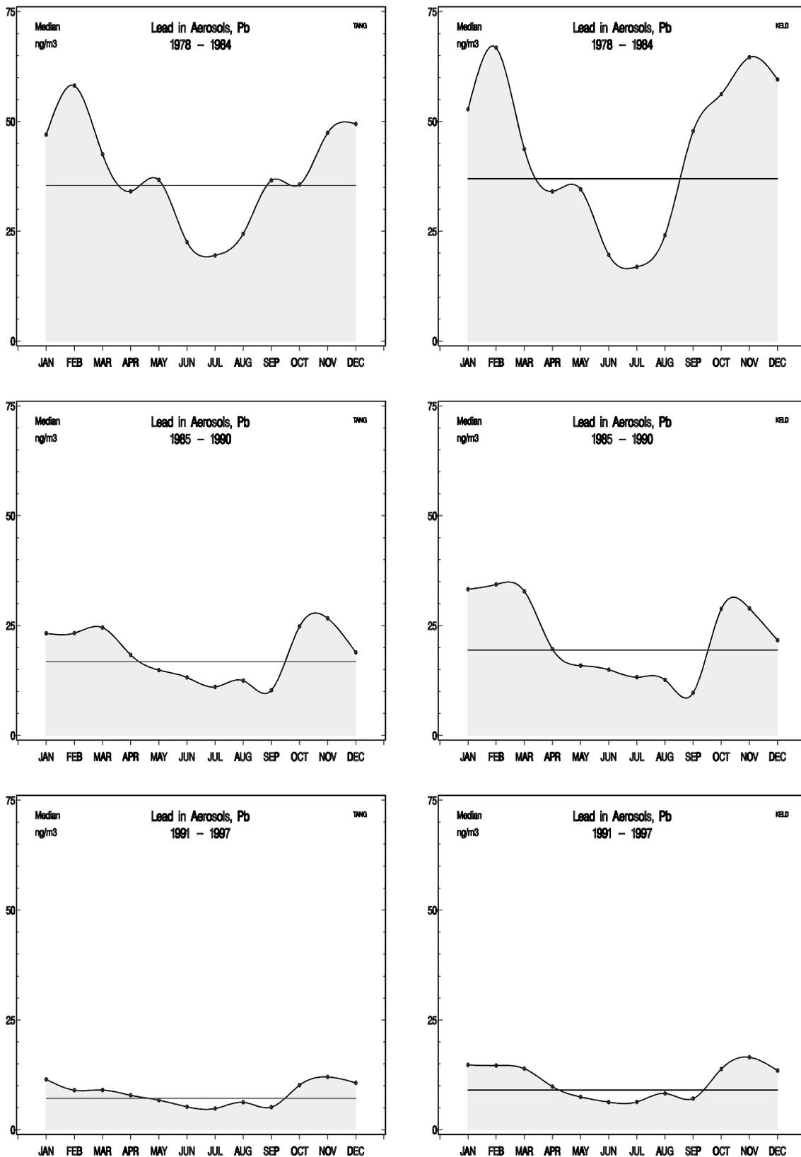
Figure 2.4.3 Average annual behaviour of monthly median concentrations of lead in aerosols in 3 subperiods. Results from station Tange at left and from Keldsnoor at right. The medians of each subperiod are shown as horizontal lines.
