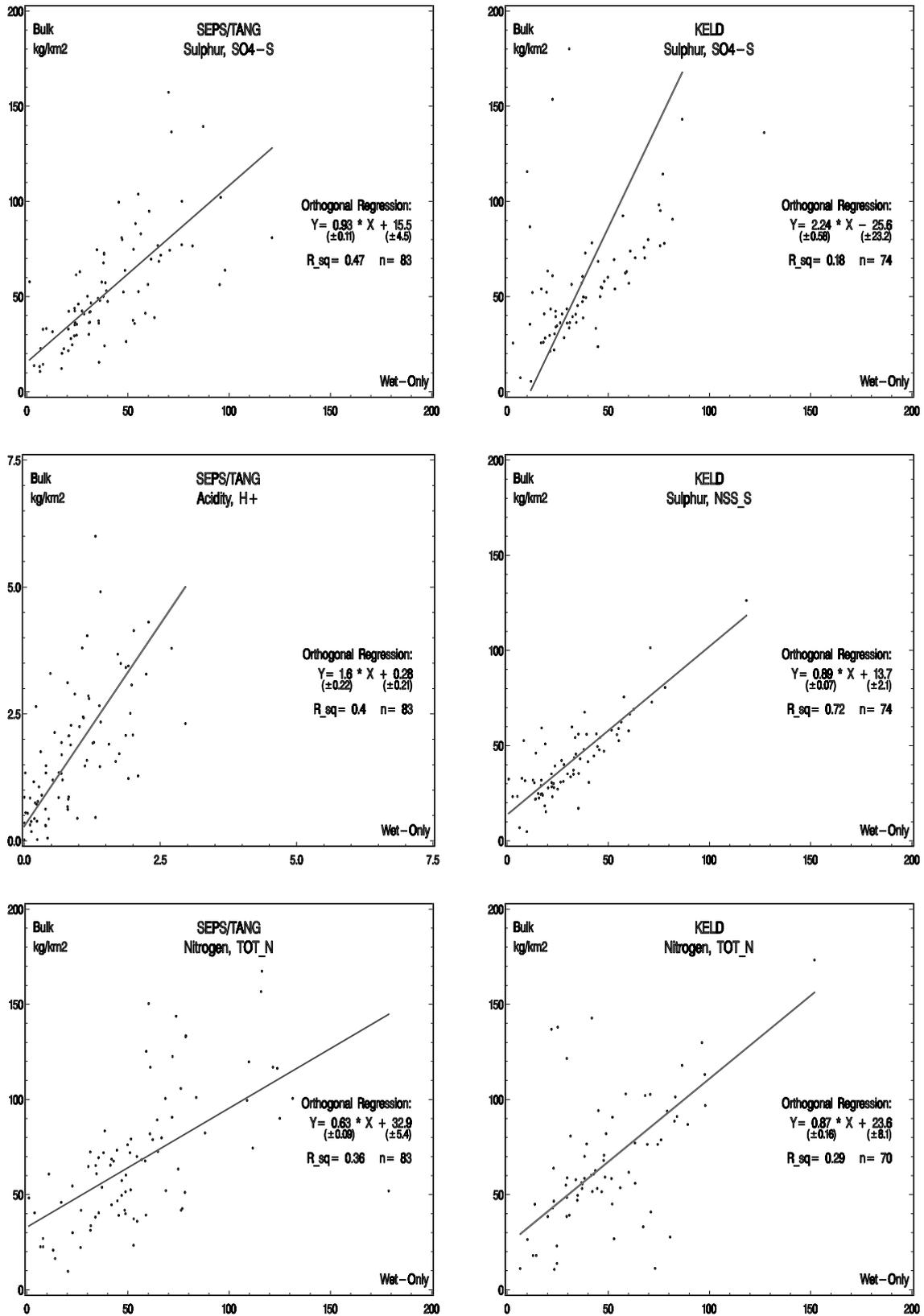
Figure 4.1.5 Monthly depositions in bulk collectors compared to wet-only samplers for the period 1991 - 1997. The results are fitted by orthogonal regression lines.
