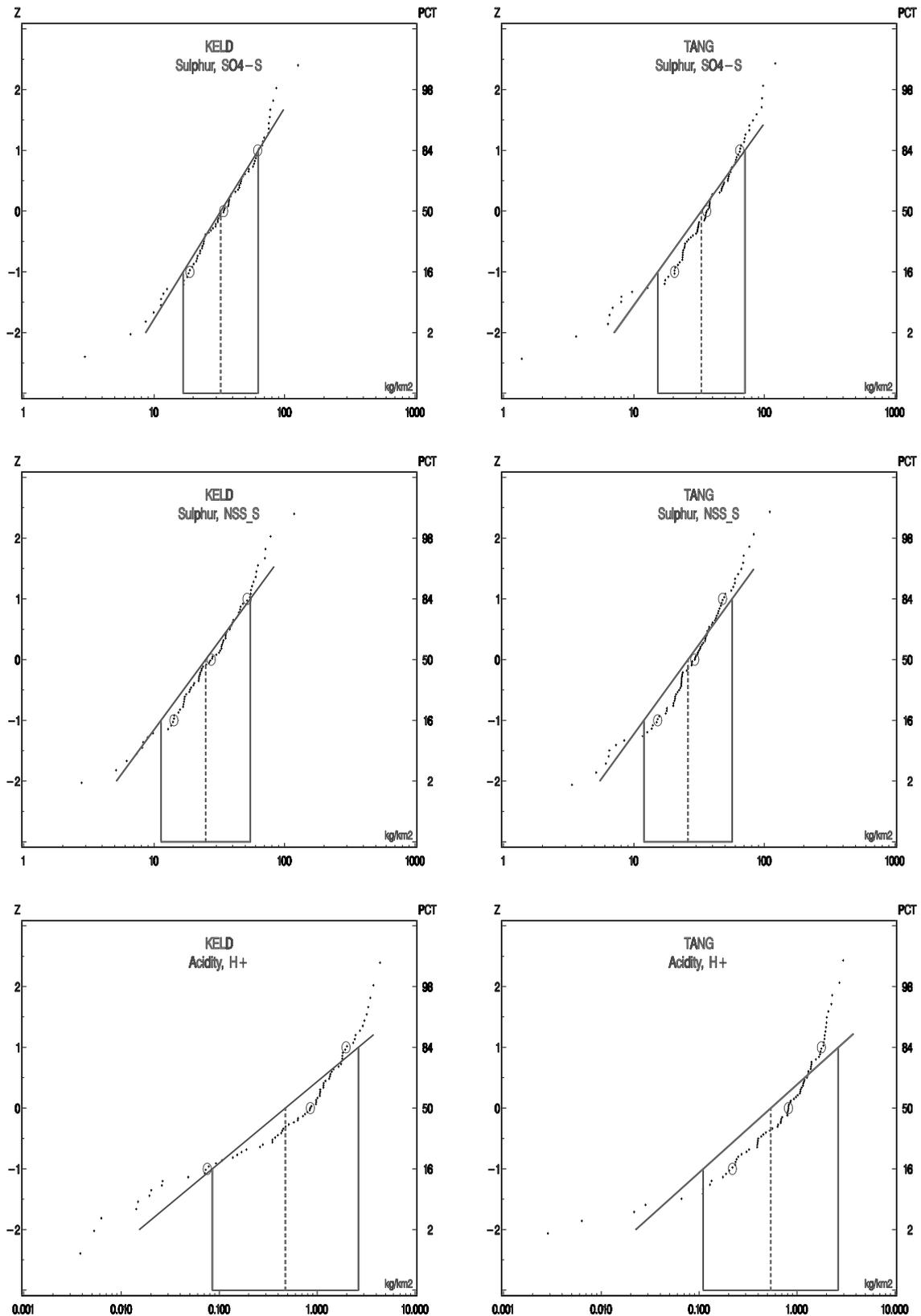
Figure 4.1.1 Statistical distributions of monthly wet-only depositions since 1991 of sulphur compounds and acidity,  $H^+$ . The depositions are shown logarithmically on the horizontal axis and circles denote the 16-, 50-, and 84-percentiles. The straight line is the log-normal fit through the indicated geometric mean and standard deviations.
