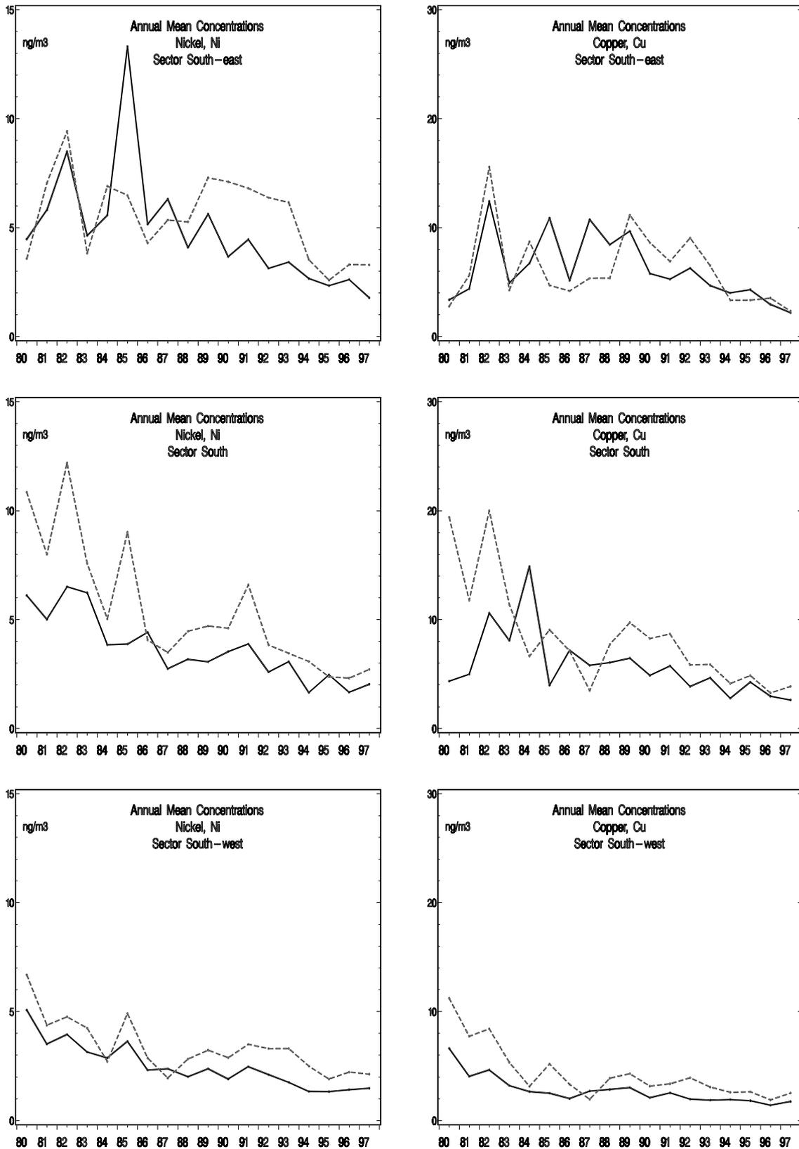
Figure 5.1.6 Annual mean concentrations of the heavy metals Ni and Cu in aerosols at Tange (full line) and Keldsnor (dashed line) in wind sectors from south-east, south, and south-west.
