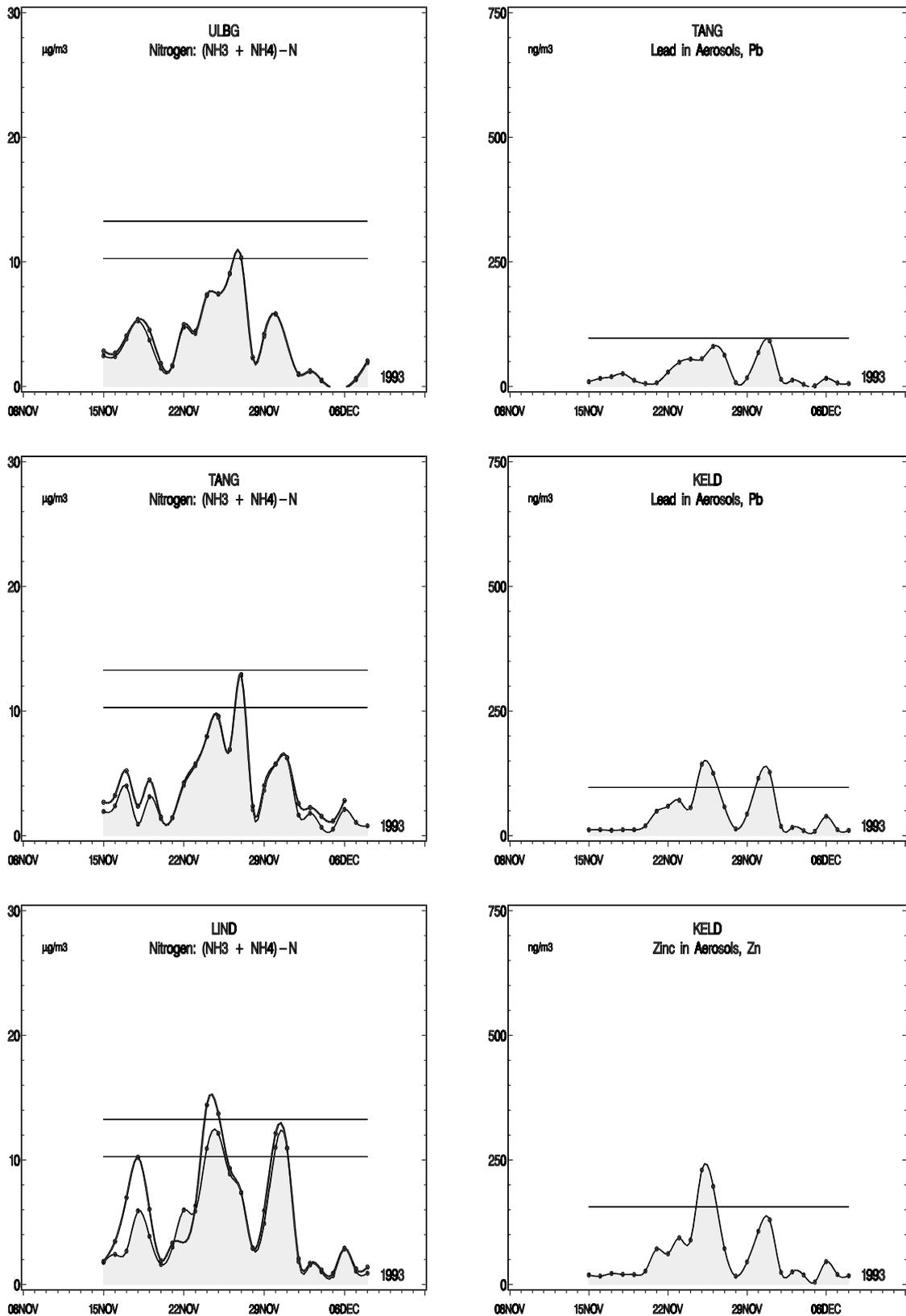
Figure 2.5.3 Episode in November 1993 with enhanced concentrations of reduced nitrogen, lead and zinc. Concentrations of total and particulate (shaded) phase on a day-by-day basis. Horizontal lines are the nation-wide 99-percentiles for particulate and total phases in 1978-1984.
