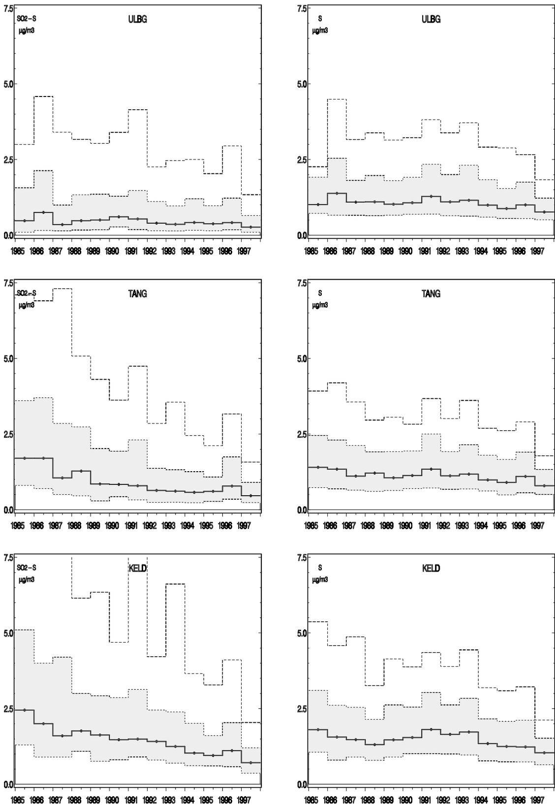
Figure 2.3.1 Annual medians, upper and lower quartiles (shaded) and the 90-percentile of 24h air concentrations of gaseous and particulate sulphur since 1985.
