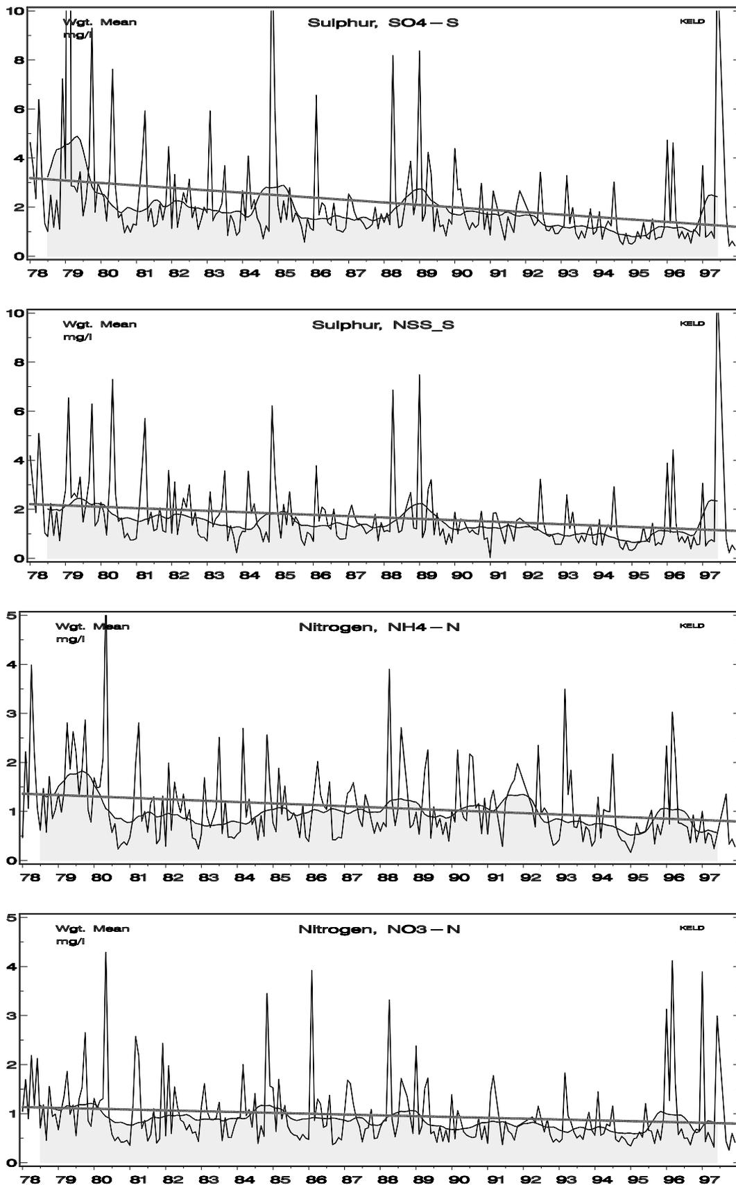
Figure 3.3.5 Trendplots for monthly precipitation weighted means at Keldsnor. The thin jagged line shows the monthly medians of the measured concentrations, the smooth curve delineating the shaded area represents a moving average over 12 months, and the full straight line is a linear regression line representing the long term trend. See also text.
