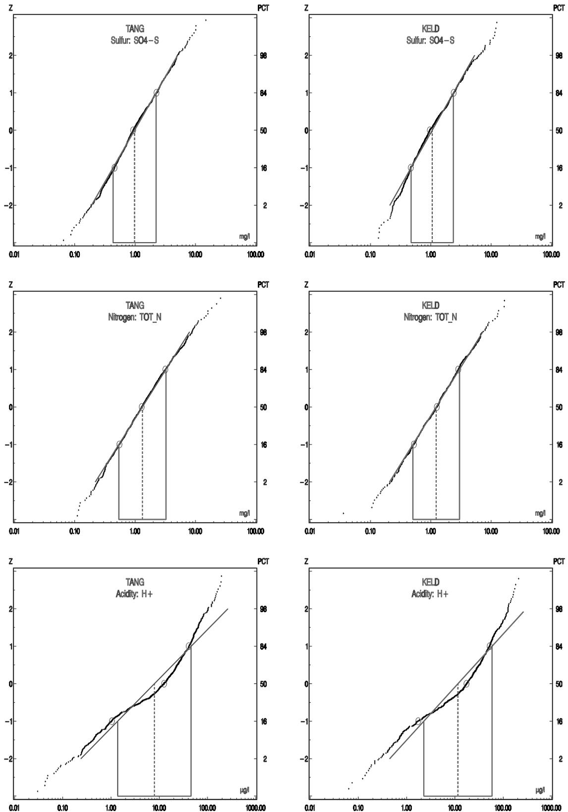
Figure 3.1.3 Statistical distributions of log-concentrations on the horizontal axis for selected pollutants in 24-h wet-only precipitation 1991-1997. Circles denote the 16-, 50-, and 84-percentiles and the straight line is the log-normal fit through the indicated geometric mean and standard deviations.
