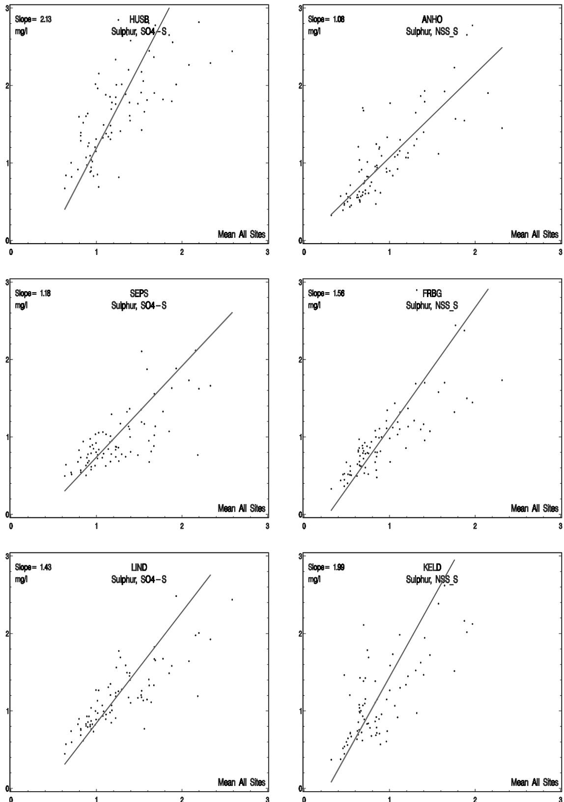
Figure 3.2.1 Monthly precipitation weighted bulk concentrations of sulphur compounds 1991- 1997. Site concentrations plotted and regressed orthogonally against the means at all sites. Calculations are based on all data, whereas displayed data amount to minimum 95% of all.
