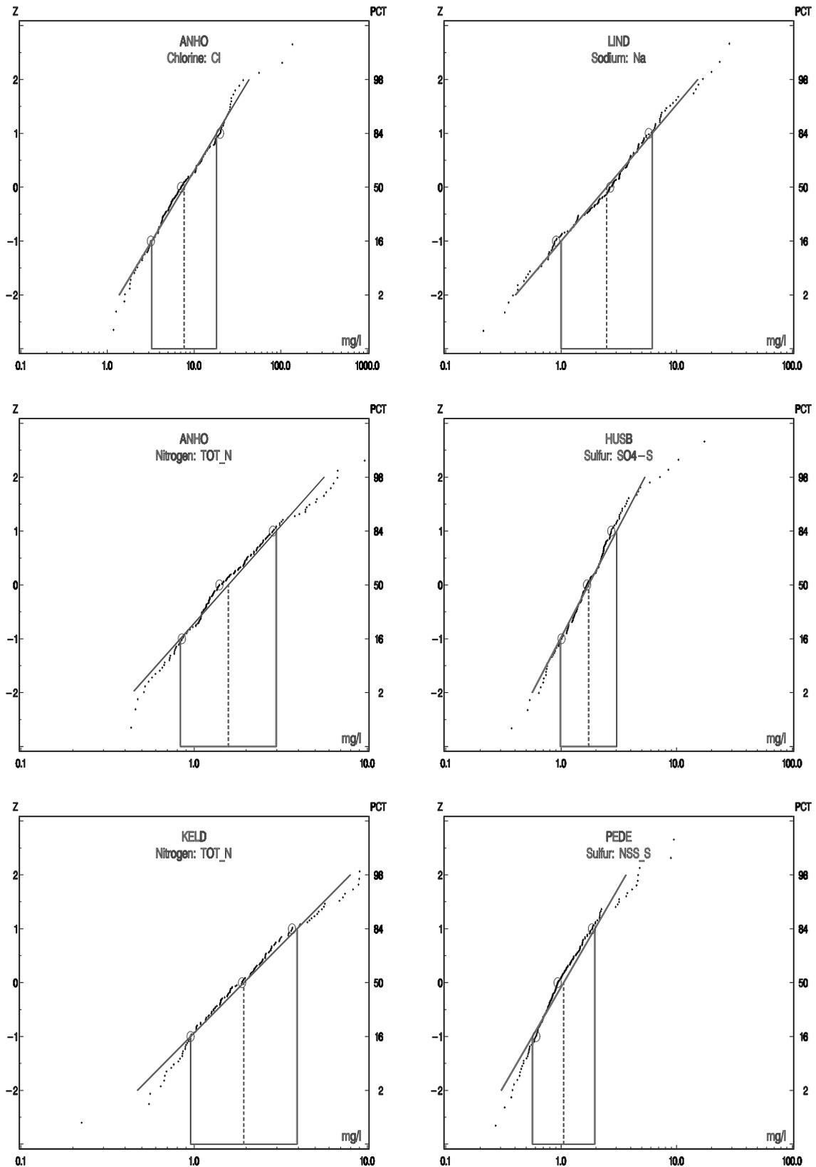
Figure 3.1.4 Statistical distributions of log-concentrations on the horizontal axis for selected pollutants in ½-monthly bulk precipitation 1991-1997. Circles denote the 16-, 50-, and 84-percentiles and the straight line is the log-normal fit through the indicated geometric mean and standard deviations.
