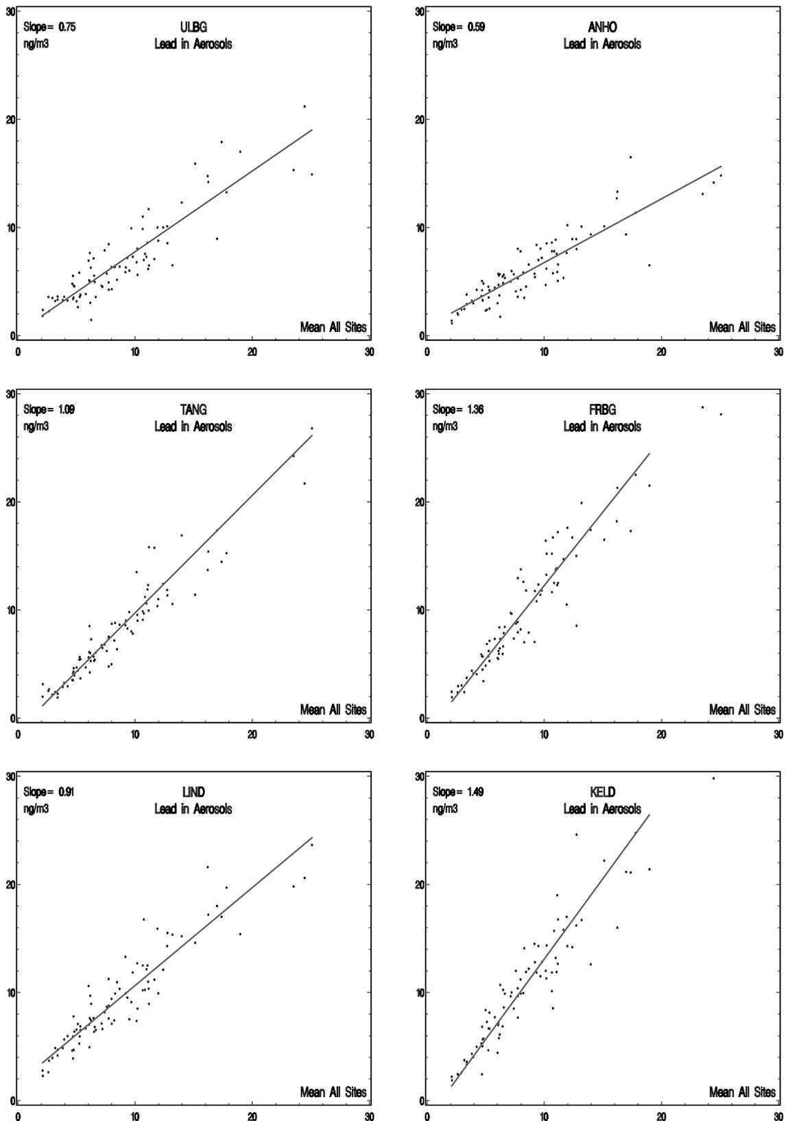
Figure 2.2.4 Monthly medians of lead in aerosols against means of monthly medians at all sites, 1991-1997, and orthogonal regressions lines.
