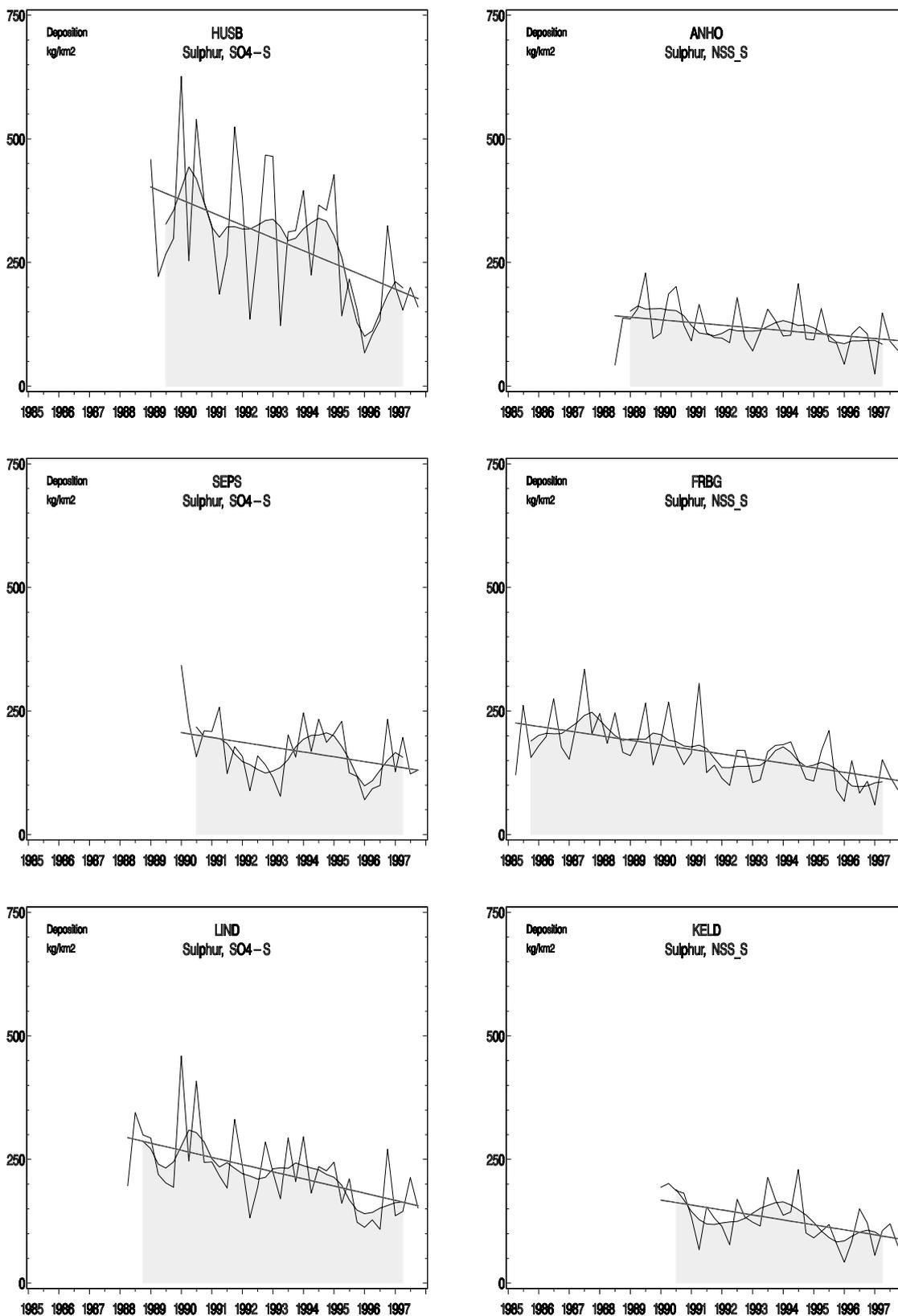
Figure 4.3.4 Quarterly bulk depositions (thin jagged line) of sulphate and NSS\_S, moving annual (4-quarter) average (shaded) and trend.
