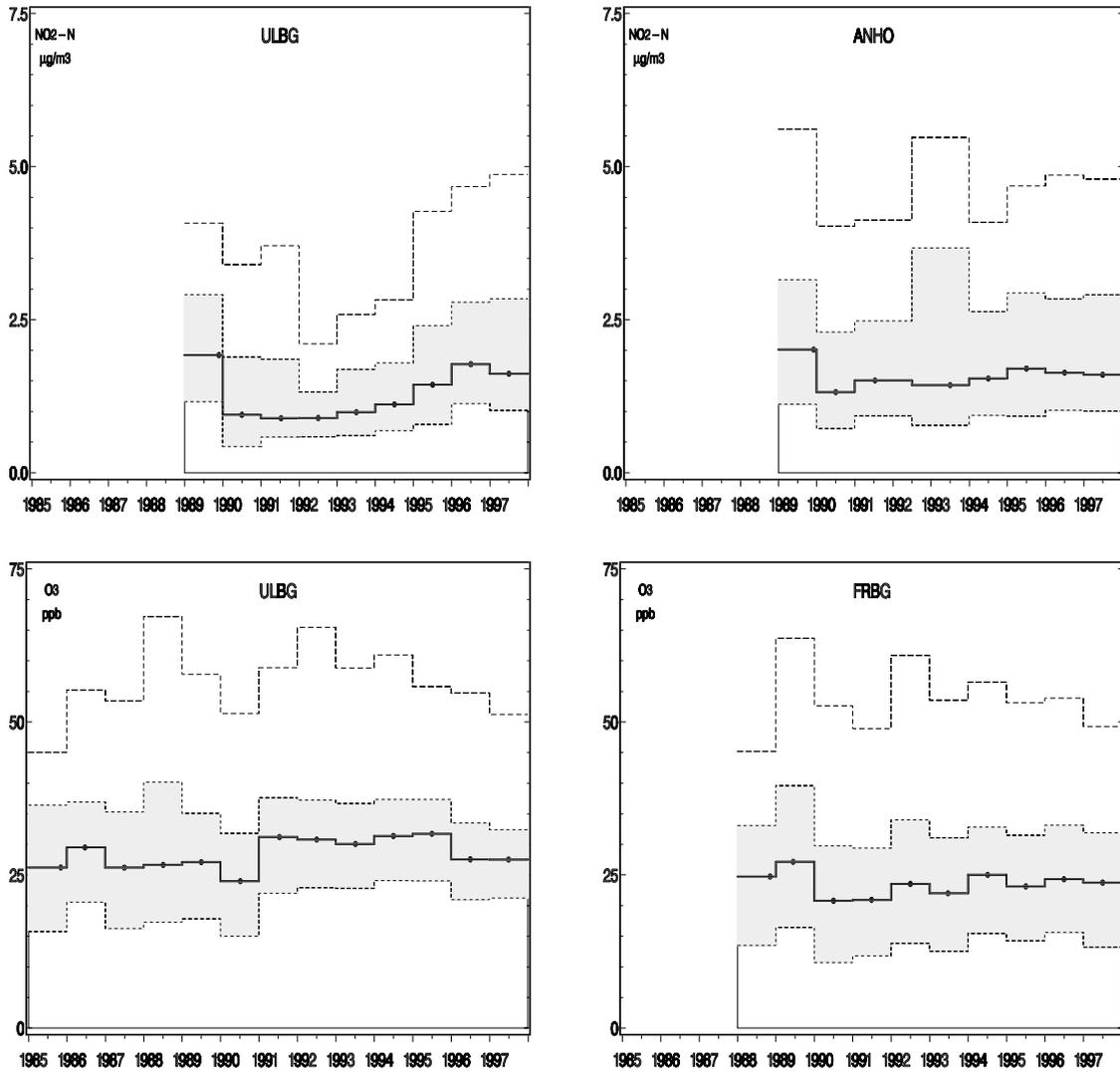
Figure 2.3.4 Annual medians and upper and lower quartiles (shaded) for 24h concentrations of NO<sub>2</sub> - N and 1h concentrations of O<sub>3</sub> since 1985. For NO<sub>2</sub> the uppermost curve is the 90-percentile and for Ozone it represents the 98-percentile.
