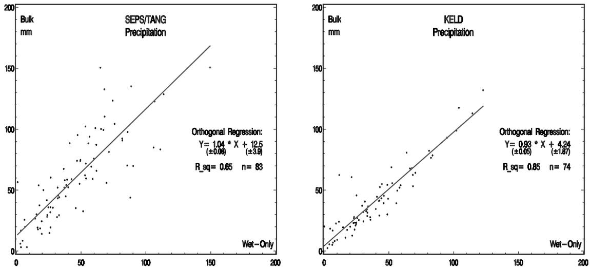
Figure 4.1.6 Monthly precipitation in bulk collectors compared to wet-only samplers for the period 1991 – 1997. The results are fitted by orthogonal regression lines.
