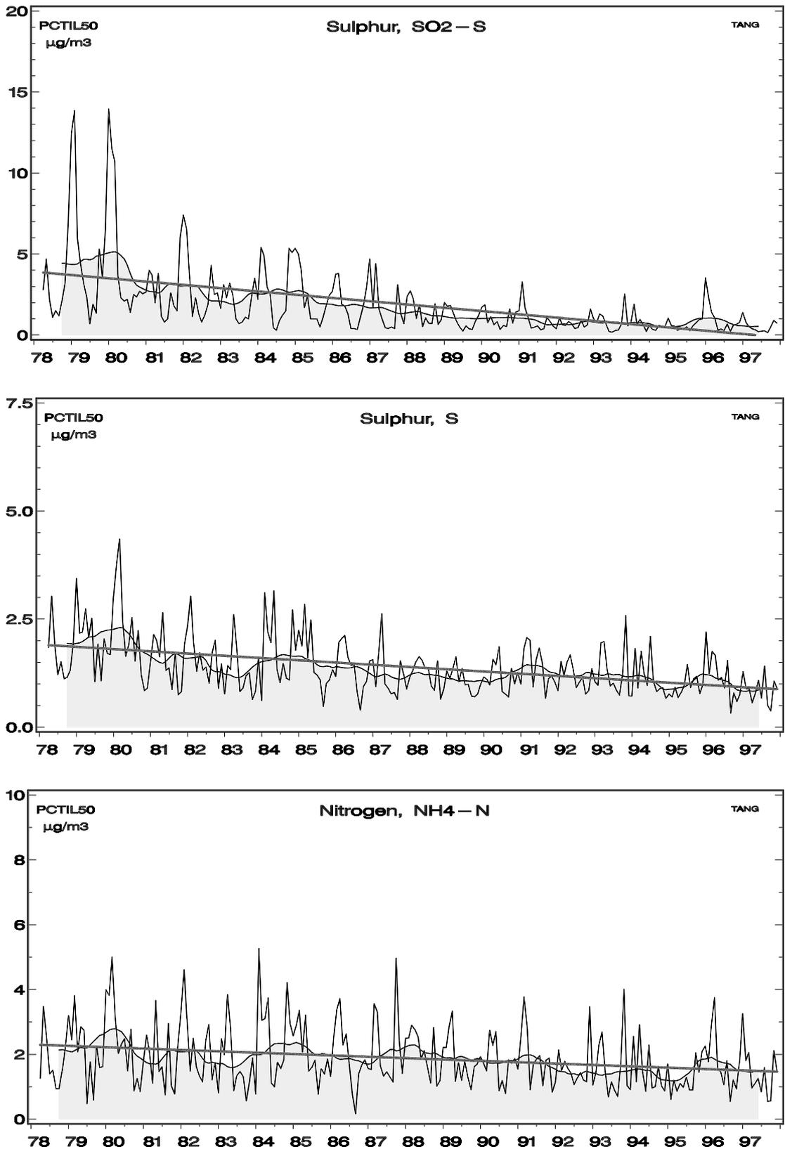
Figure 2.3.5 Trends for monthly medians of SO<sub>2</sub>-S, particulate S, and NH<sub>4</sub>-N at Tange. The thin jagged line shows the monthly medians of the measured concentrations, the smooth curve delineating the shaded area represents a moving average over 12 months, and the full straight line is a linear regression line representing the long term trend. See also text.
