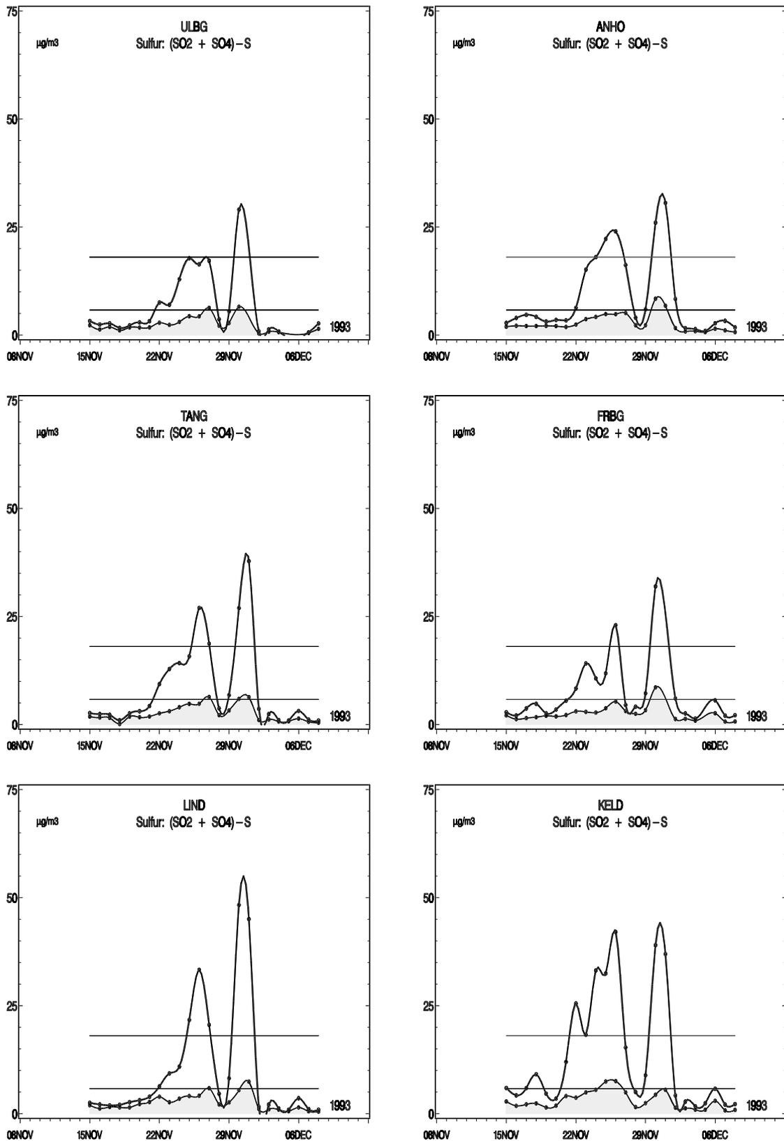
Figure 2.5.2 Episode in November 1993 with enhanced sulphur concentrations at all stations. Concentrations of total and particulate (shaded) phase on a day-by-day basis. Horizontal lines are the nation-wide 99-percentiles for particulate and total phases in 1978-1984.
