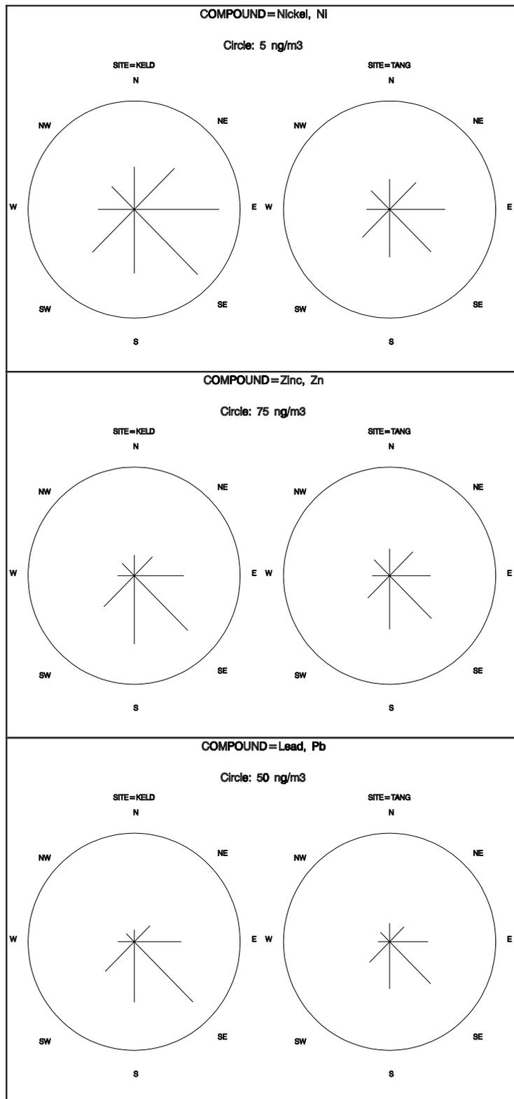
Figure 5.1.2 Mean concentrations of Nickel, Zinc, and Lead in aerosols at Keldsnor and Tange for 1991 - 1997. The sector value is the mean concentration in winds from that direction. For each compound the scale is given by the radius of the circumscribing circle.
