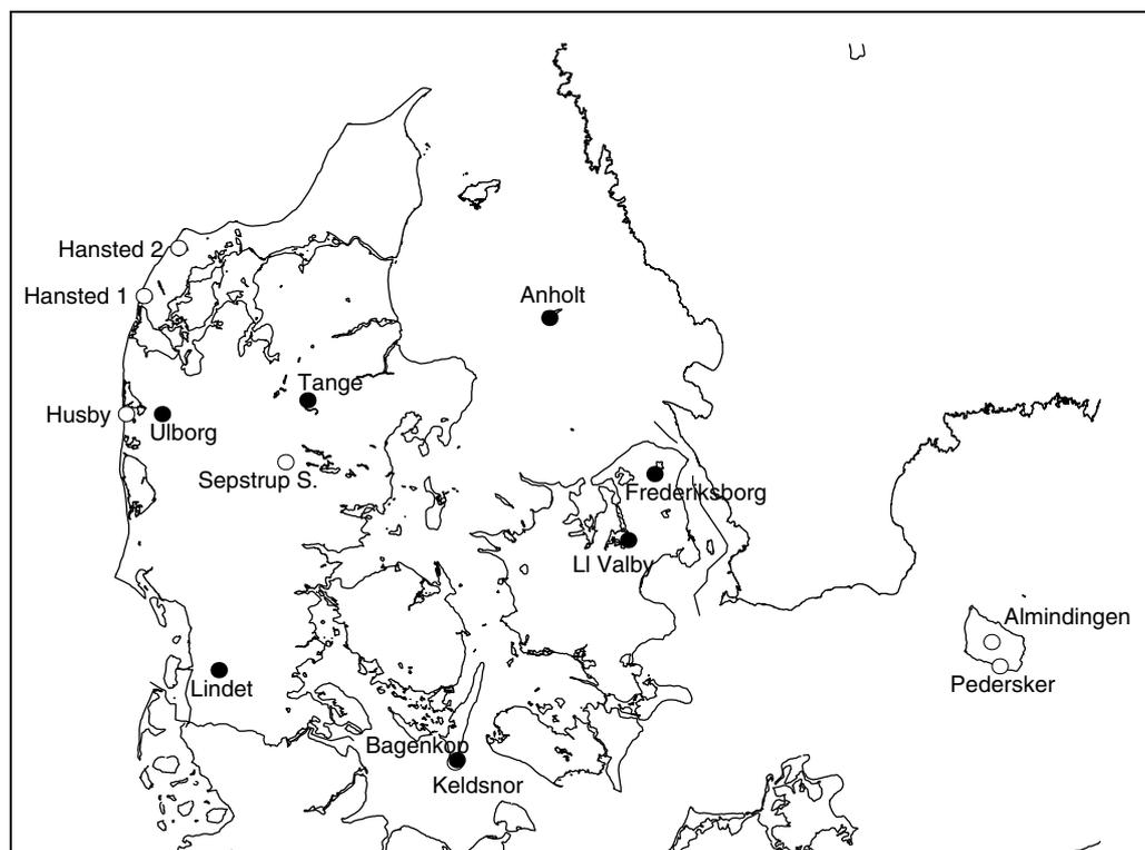
Figure 1.2.1 Map of the BOP stations in Denmark in 1996 - 1997. ● Main stations with measurements of gases and aerosols and wet-only collection of precipitation. ○ Substations with bulk sampling of precipitation.
