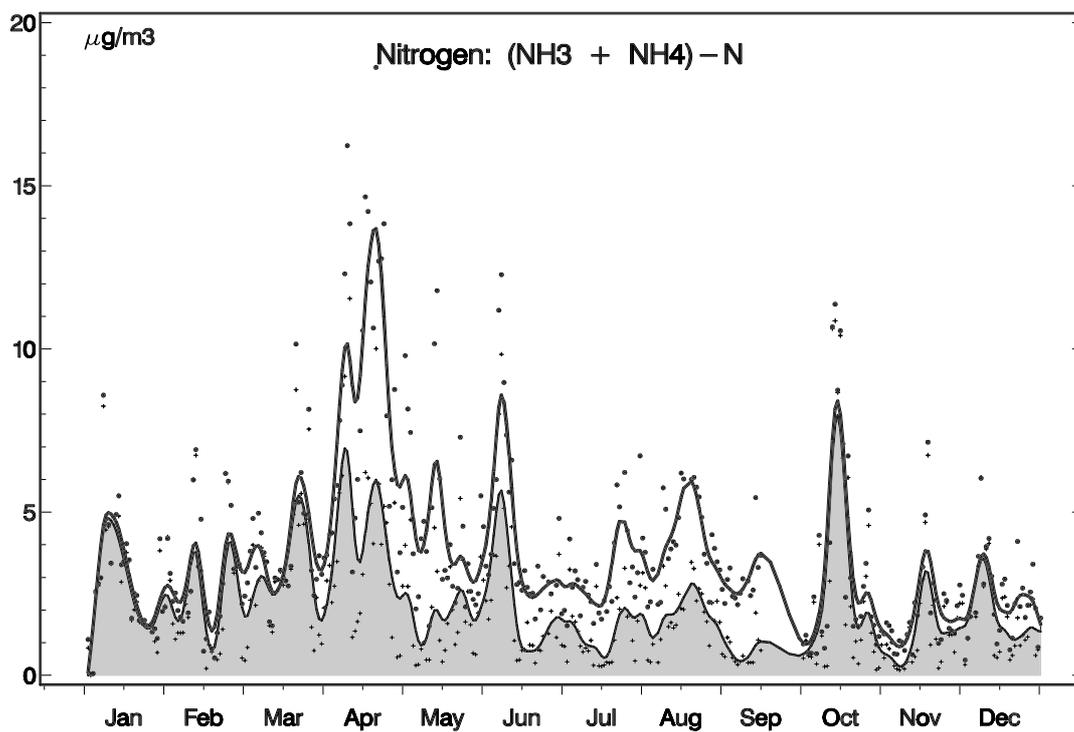
Figure 2.1.1 Daily concentrations in air (points) of sulphur and reduced nitrogen compounds at Tange in 1996, overlaid with smoothing curves. Concentrations of gaseous (dots) and particulate phases (crosses, shaded) are summed.
