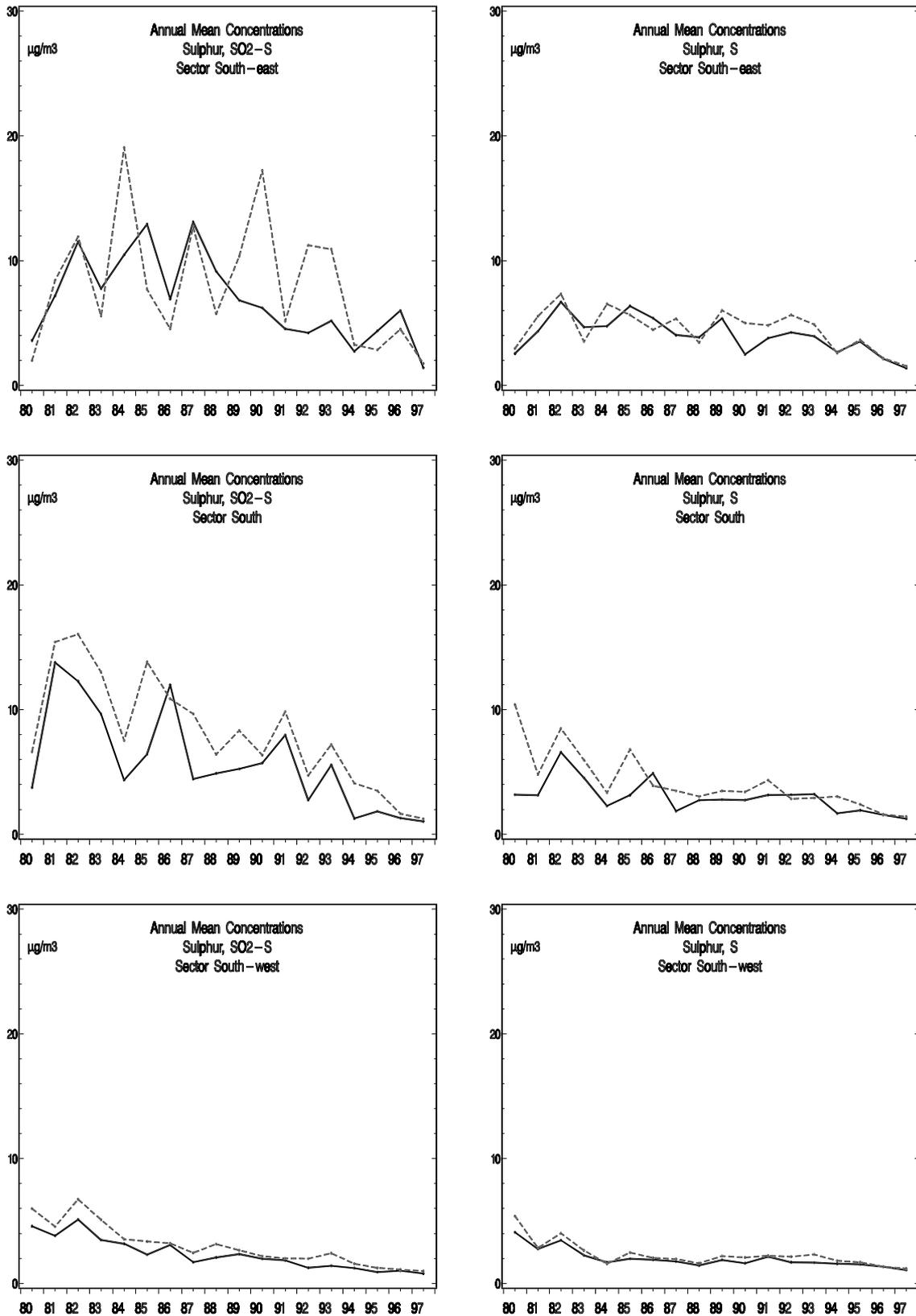
Figure 5.1.5 Annual mean concentrations of  $\text{SO}_2$  and S at Tange (full line) and Keldsnor (dashed line) in wind sectors from south-east, south, and south-west.
