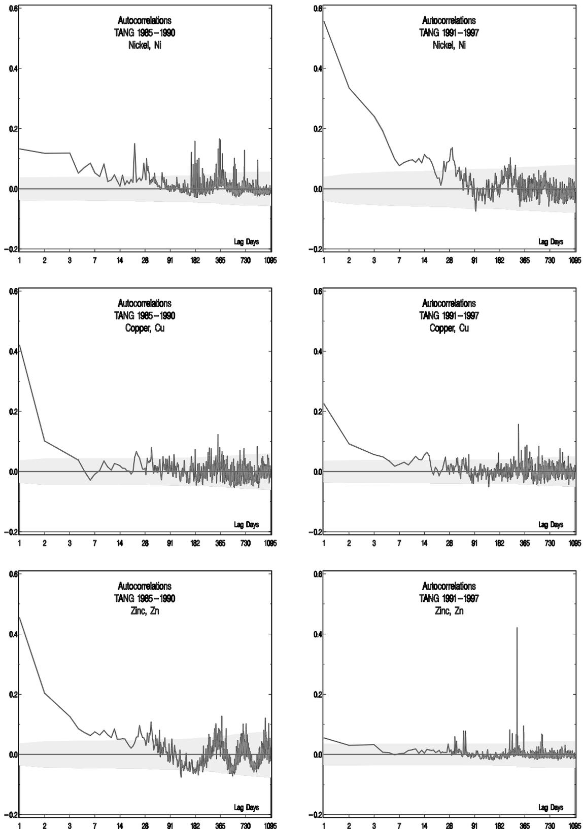
Figure 2.1.8 Autocorrelation functions over 3 years for some heavy metal concentrations at Tange in 1985-1990 and 1991-1997. Values outside the shaded area are significant at the 5%-level.
