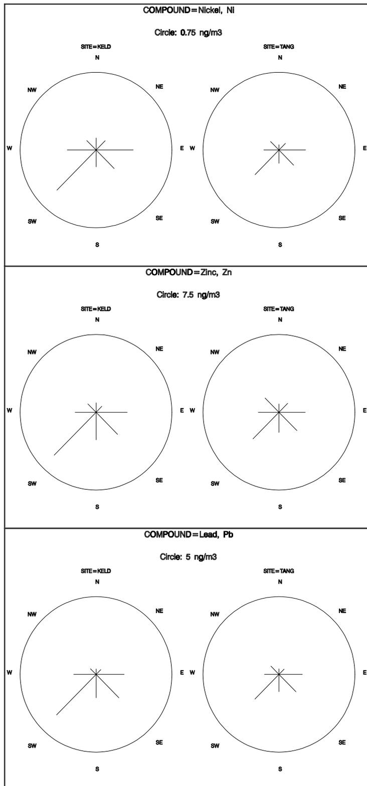
Figure 5.1.4 Wind frequency weighted mean concentrations of Nickel, Zinc, and Lead in aerosols at Keldsnor and Tange for 1991 - 1997. The sector value is equal to the contribution from that sector to the overall mean value for the period. For each compound the scale is given by the radius of the circumscribing circle.
