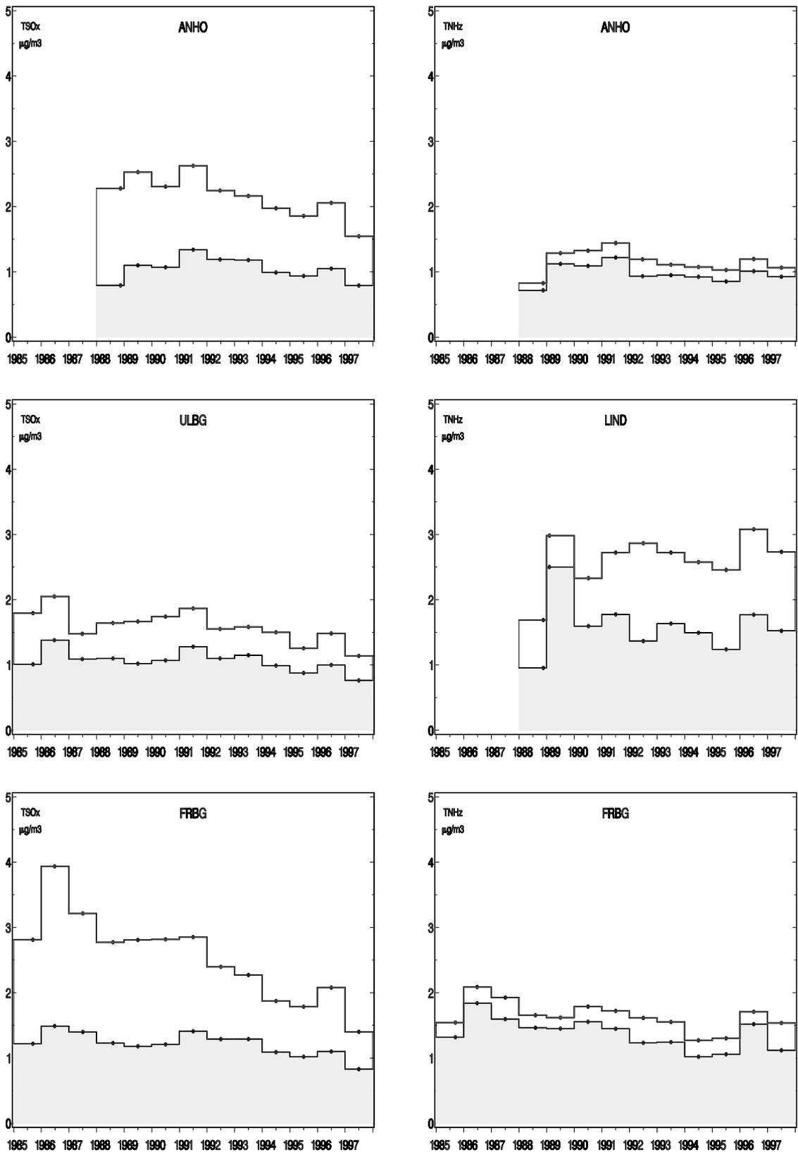
Figure 2.2.2 Annual medians of 24h concentrations of compounds of sulphur (left) and reduced nitrogen (right), split into gaseous phases  $\text{SO}_2$ -S and  $\text{NH}_3$ -N (blank) and particulate phases S, including  $\text{SO}_4^{2-}$ -S, and  $\text{NH}_4^+$ -N (shaded).
