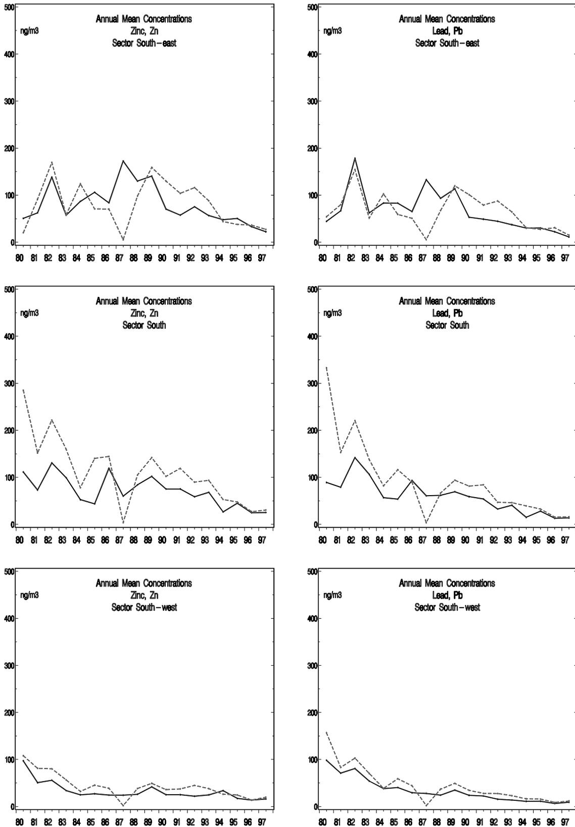
Figure 5.1.7 Annual mean concentrations of the heavy metals Zn and Pb in aerosols at Tange (full line) and Keldsnor (dashed line) in wind sectors from south-east, south, and south-west.
