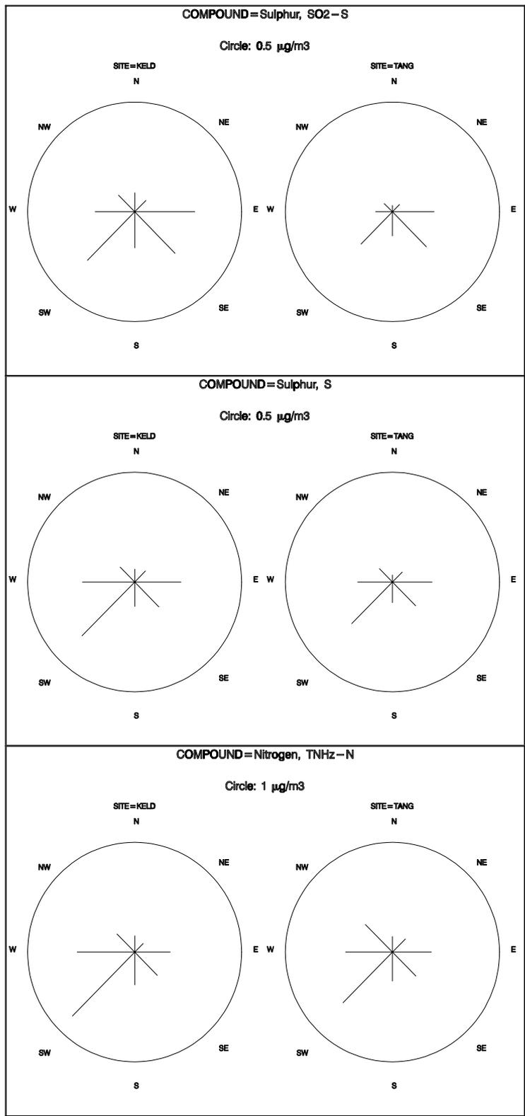
Figure 5.1.3 Wind frequency weighted mean concentrations of SO<sub>2</sub>, S and TNHz at Keldsnoor and Tange for 1991 - 1997. The sector value is equal to the contribution from that sector to the overall mean value for the period. For each compound the scale is given by the radius of the circumscribing circle.
