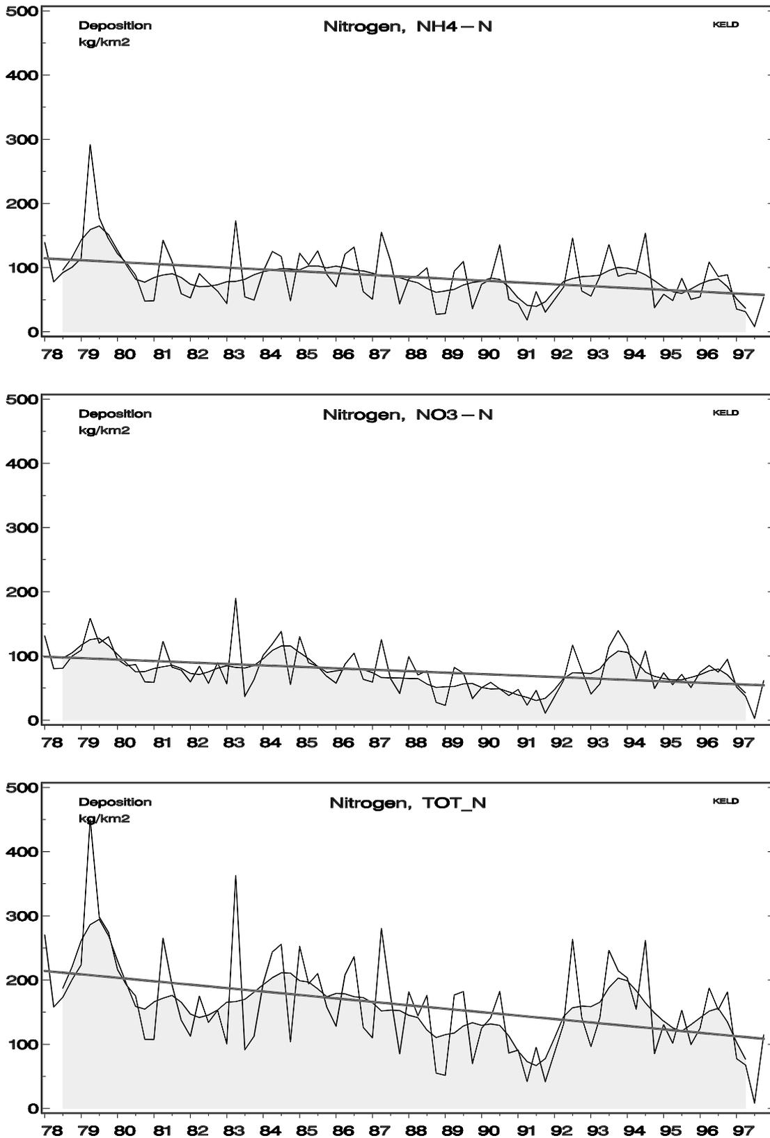
Figure 4.3.8 Quarterly wet-only depositions (thin jagged line) of nitrogen compounds at Keldsnoor 1978 - 1997, moving annual average (shaded) and trend.
