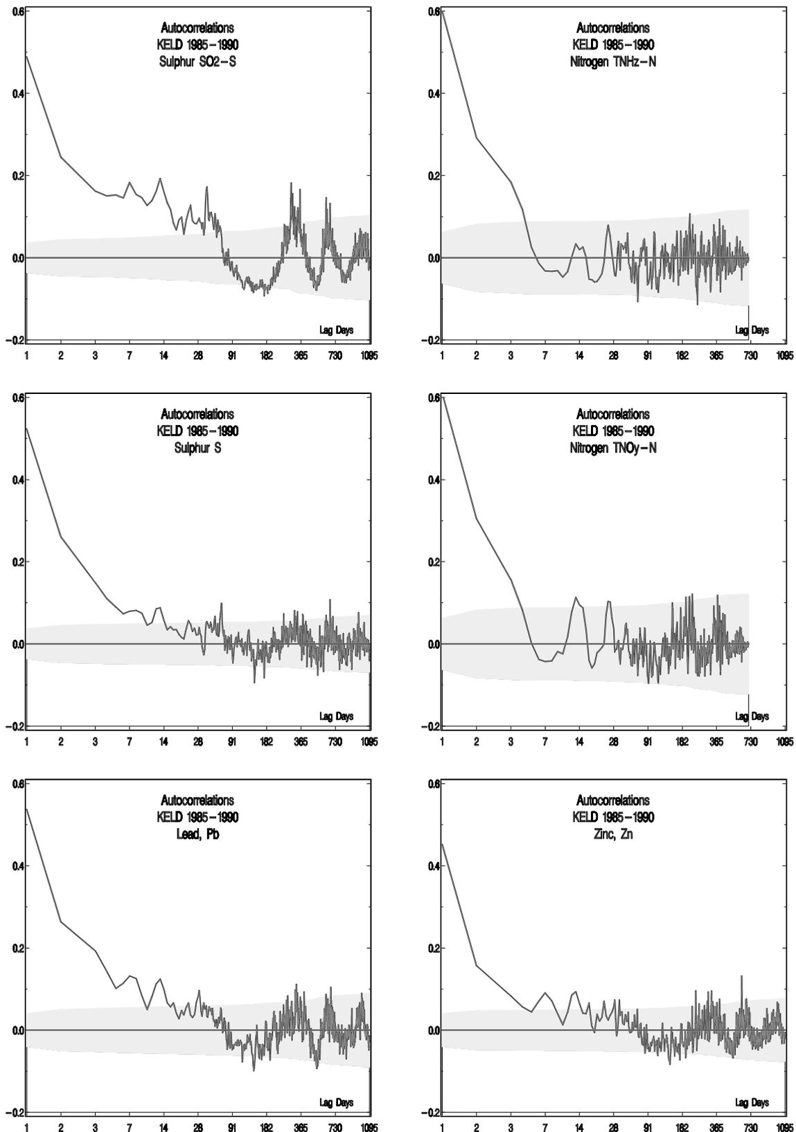
Figure 2.1.7 Autocorrelation functions over 3 years for concentrations of selected pollutants at Keldsnoor 1985-1990. Values outside the shaded area are significant at the 5%-level.
