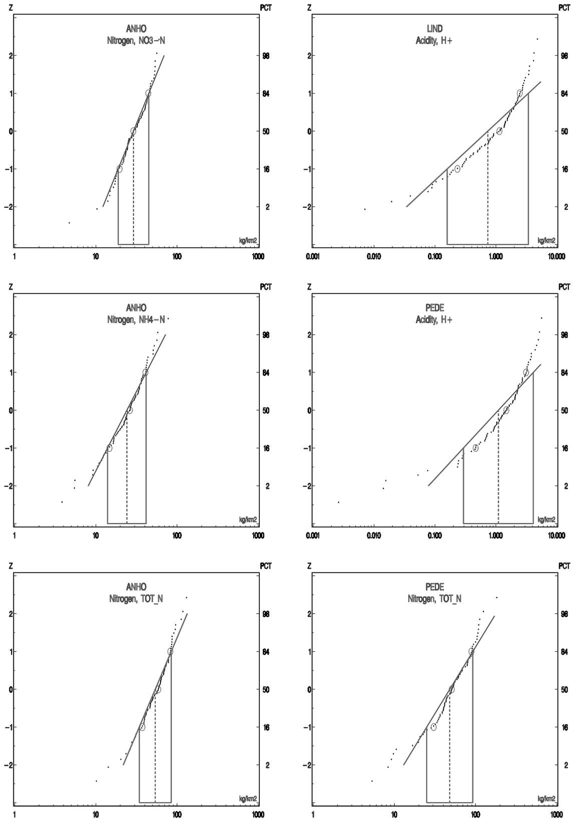
Figure 4.1.4 Statistical distributions of monthly bulk depositions since 1991 of nitrogen compounds and acidity, H<sup>+</sup>. The depositions are shown logarithmically on the horizontal axis and circles denote the 16-, 50-, and 84-percentiles. The straight line is the log-normal fit through the indicated geometric mean and standard deviations.
