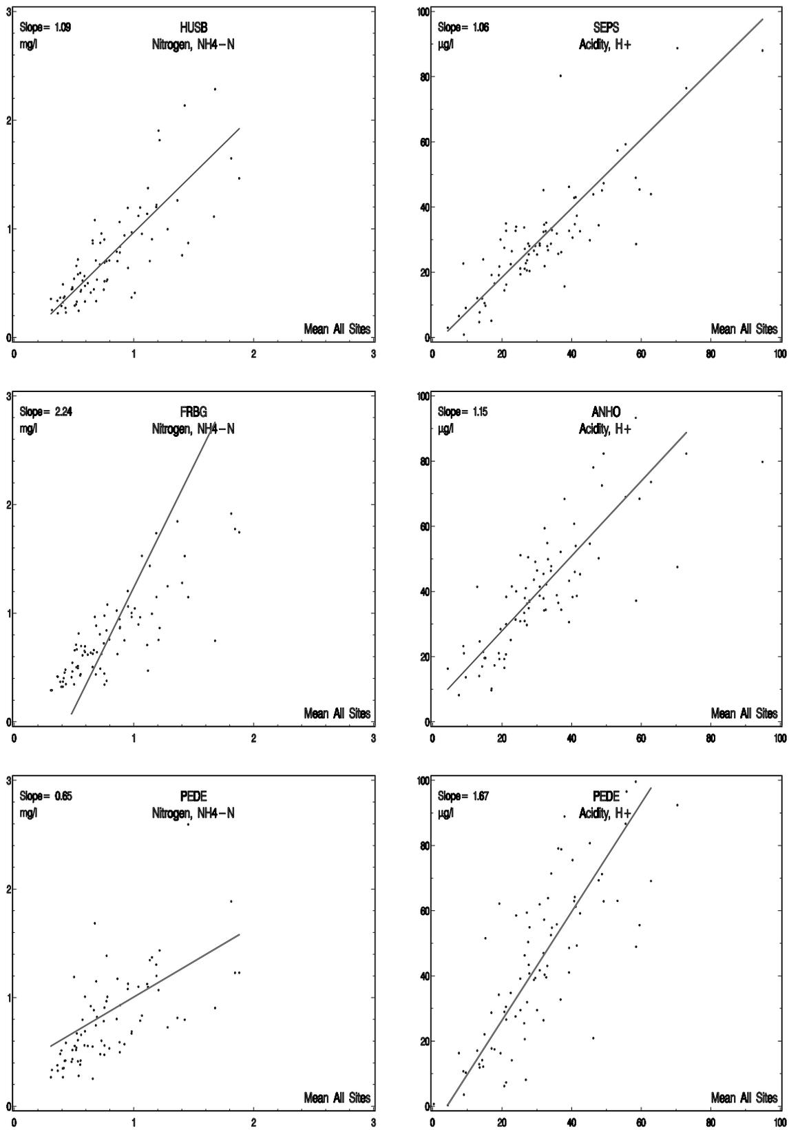
Figure 3.2.3 Monthly precipitation weighted bulk concentrations of nitrogen compounds and acidity 1991-1997. Site concentrations plotted and regressed orthogonally against the means at all sites. Calculations are based on all data, whereas displayed data amount to minimum 95% of all.
