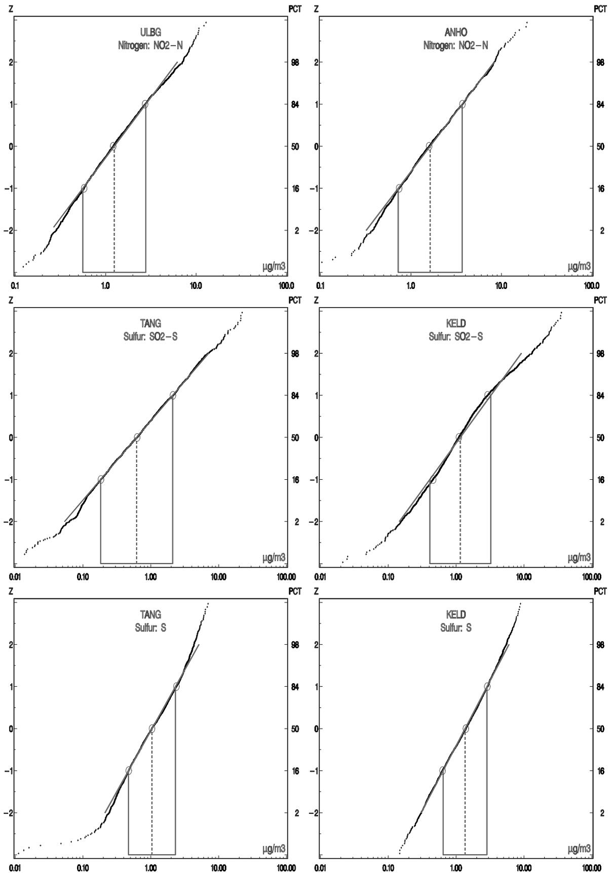
Figure 2.1.4 Statistical distributions of log-concentrations on the horizontal axis for selected pollutants and stations in 1991-1997. Circles denote the 16-, 50-, and 84-percentiles and the straight line is the log-normal fit through the indicated geometric mean and standard deviations. See also text.
