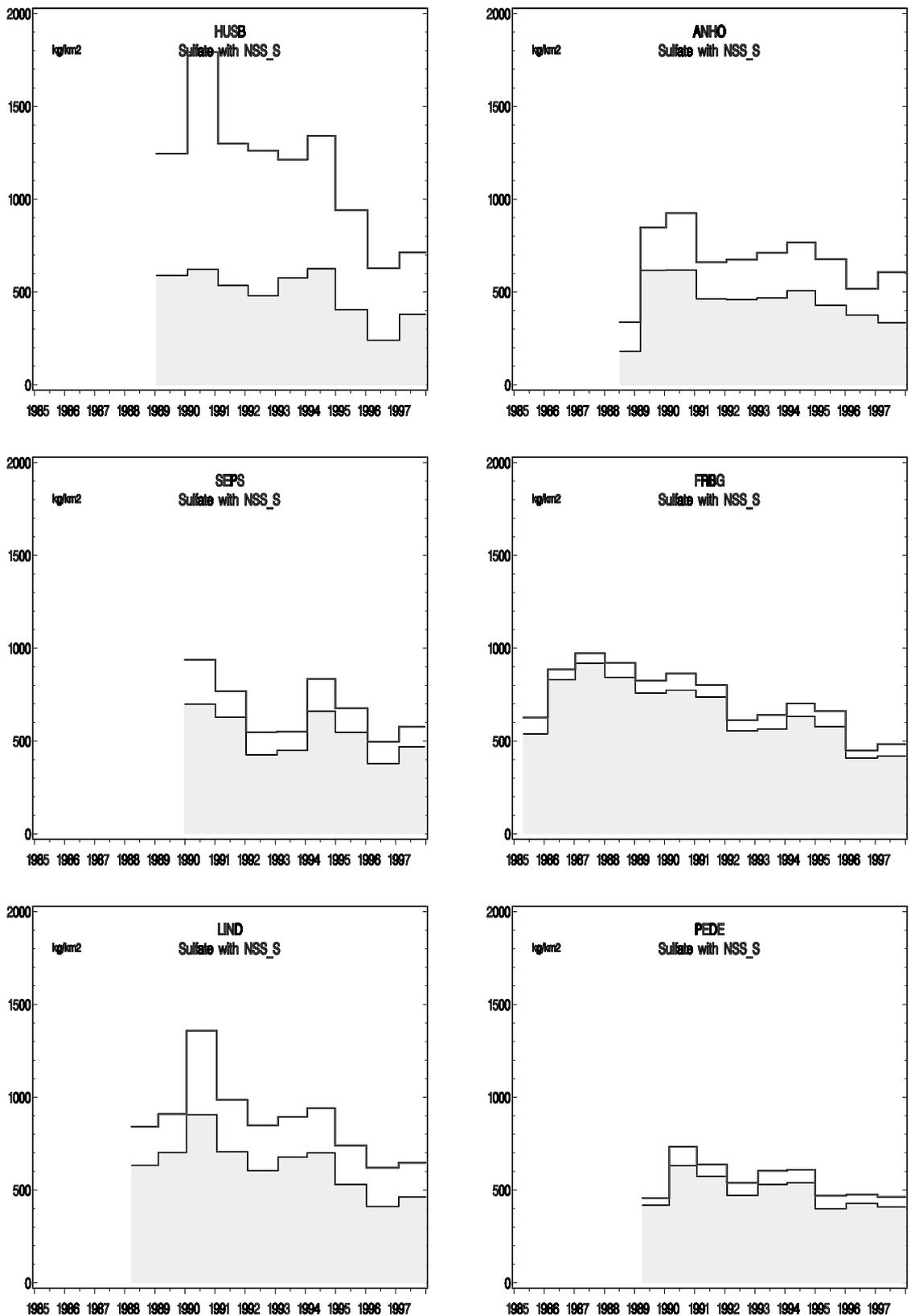
Figure 4.3.1 Annual bulk depositions of sulphate, SO<sub>4</sub> and the fraction of NSS\_S (shaded) in kg S/km<sup>2</sup>, 1985 - 1997.
