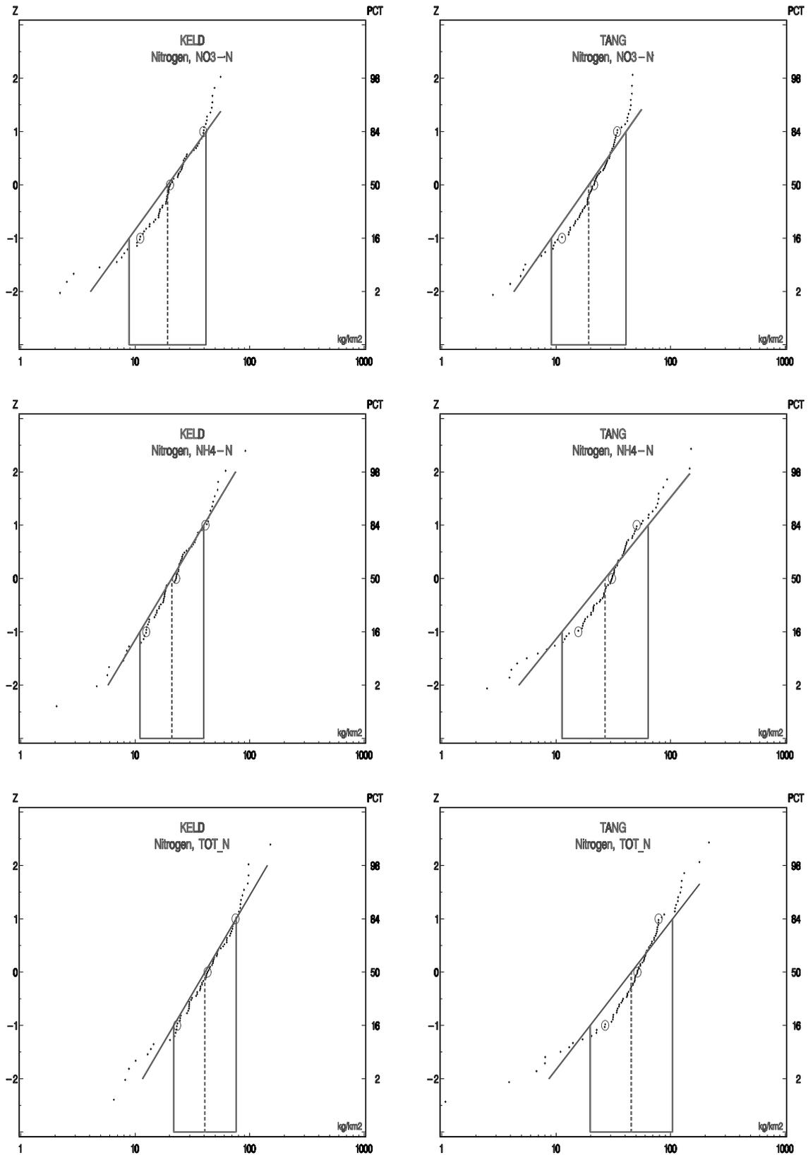
Figure 4.1.2 Statistical distributions of monthly wet-only depositions since 1991 of nitrogen compounds. The depositions are shown logarithmically on the horizontal axis and circles denote the 16-, 50-, and 84-percentiles. The straight line is the log-normal fit through the indicated geometric mean and standard deviations.
