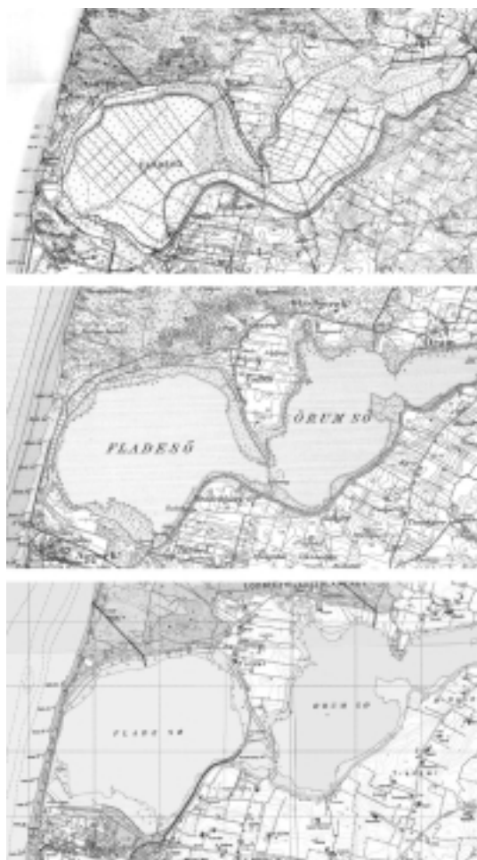
Figure 6. During 1868-1875 the lake basin of Lake Flade-Ørum was drained to create farmland (map at top, Høje Målebordsblade M20, 1871-1883, © Kort og Matrikelstyrelsen). Around 1882, the land reclamation was abandoned and Lake Flade-Ørum re-established (map in the middle, Topografisk Kort A1402, 1917, © Kort og Matrikelstyrelsen). In the mid-1950s, embankments were built isolating Lake Flade-Ørum into the present-day Lake Flade (4.3 km 2 ), Lake Ørum (4.3 km 2 ) and Lake Roddenbjerg (0.2 km 2 ) (map at the bottom, Danmarks Topografiske Kortværk 2000 © Kort og Matrikelstyrelsen).
