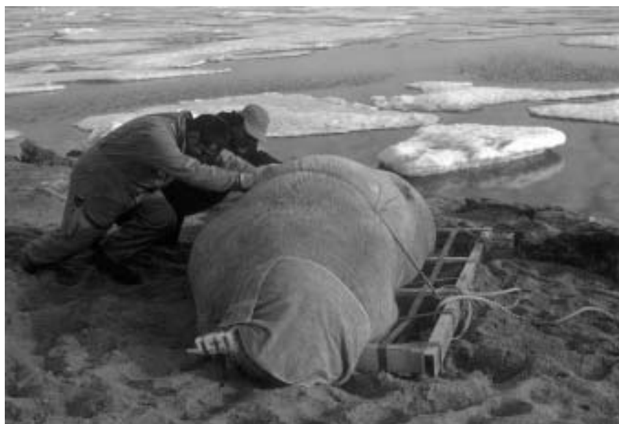
Figure 7 Weighing system used in NE Greenland 2000-2001. The immobilized walrus is rolled onto an aluminum rack resting on 4 load cells (photo: M.Acquarone).
