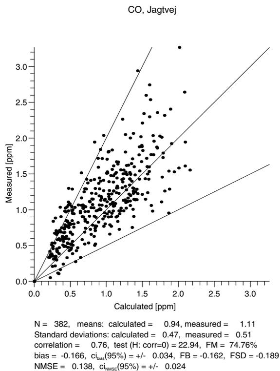
Figure 19d. Comparisons of measurements and the daily mean values of the 12 hours forecasted CO modelled concentrations at Jagtvej, Copenhagen, Denmark for the period August 1998 to September 1999.
