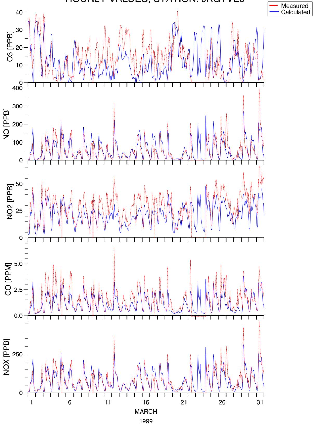
Figure 18. Comparisons of hourly values of measurements (red curves) and 12 hours forecasts using the OSPM model (blue curves) for March 1999 at Jagtvej (eastern side), Copenhagen, Denmark.
