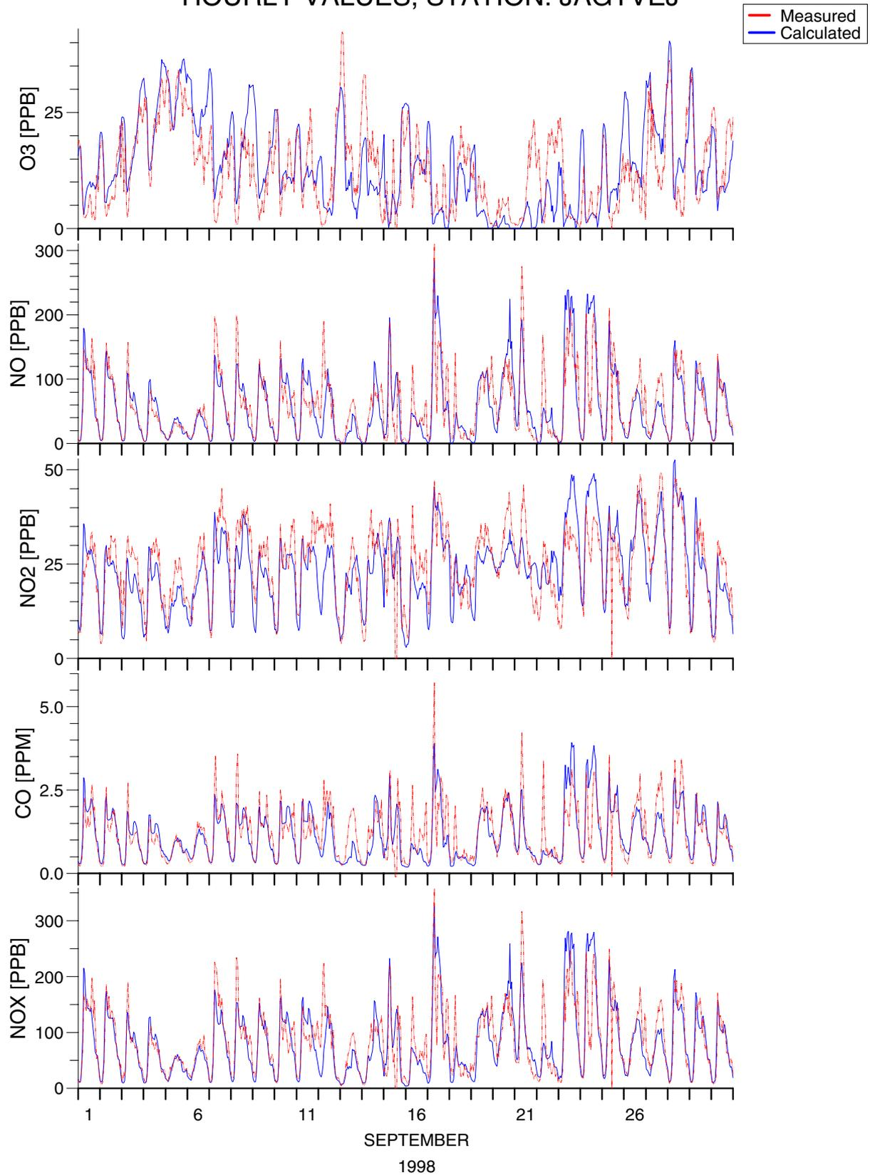
Figure 16. Comparisons of hourly values of measurements (red curves) and 12 hours forecasts using the OSPM model (blue curves) for September 1998 at Jagtvej (eastern side), Copenhagen, Denmark.
