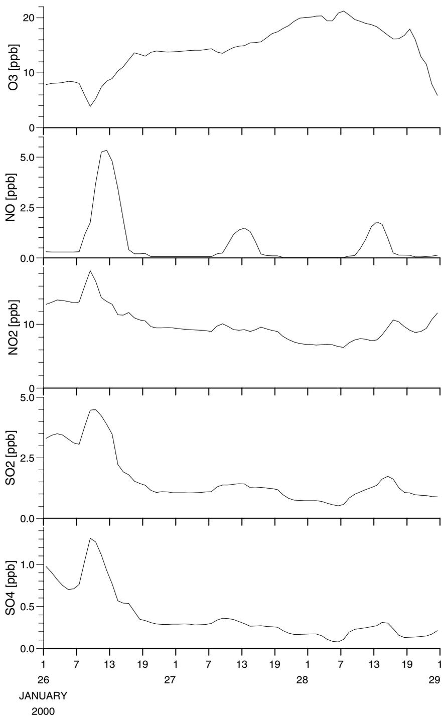
Figure 10. Time series of forecasted regional concentrations of O<sub>3</sub>, NO, NO<sub>2</sub>, SO<sub>2</sub> and SO<sub>4</sub> over Copenhagen, for the period January 26<sup>th</sup>, 00 UTC, to January 29<sup>th</sup>, 00 UTC, 2000. Results are calculated using the regional air pollution model, DEOM.
