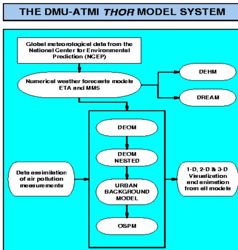
Figure 21a. schematic diagram of the future main modules and the data flow in the DMU-ATMI THOR air pollution forecast system.
