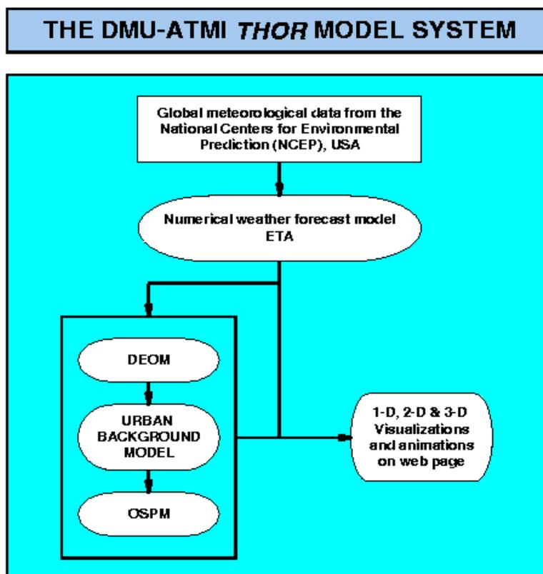
Figure 1. A schematic diagram of the main modules and the data flow in the DMU-ATMI THOR air pollution forecast system.
