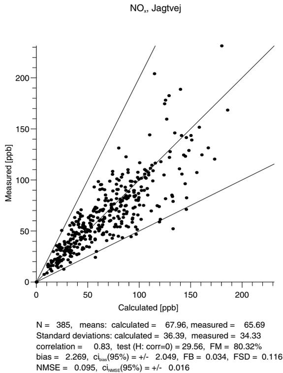
Figure 19c. Comparisons of measurements and the daily mean values of the 12 hours forecasted NO<sub>x</sub> modelled concentrations at Jagtvej, Copenhagen, Denmark for the period August 1998 to September 1999.
