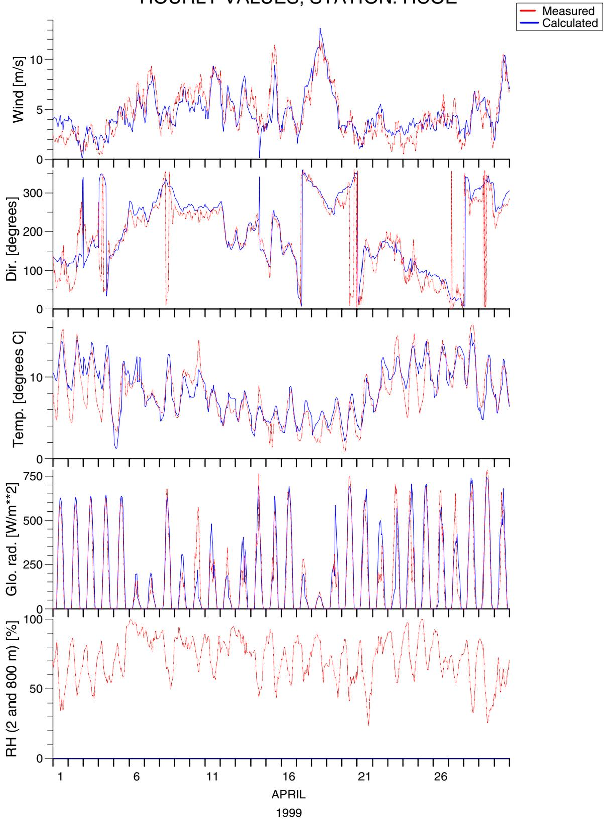
Figure 15. Comparisons of hourly values of measurements (red curves) and 12 hours forecasts using the ETA model (blue curves) for April 1999 at HCØ (roof), Copenhagen, Denmark, (only model results are shown for the relative humidity).
