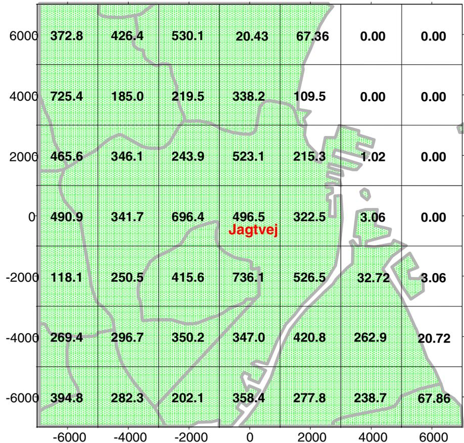
Figure 4. Average daily emissions of  $\text{NO}_x$  in Copenhagen (in kg/grid/day). Units in the x- and y-axes are distance in m from the centre of the grid (Berkowicz, 1999b).
