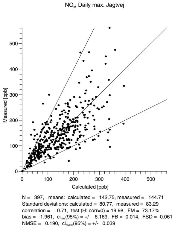
Figure 20c. Comparisons of measurements and the daily maximum values of the 12 hours forecasted NO<sub>x</sub> modelled concentrations at Jagtvej, Copenhagen, Denmark for the period August 1998 to September 1999.
