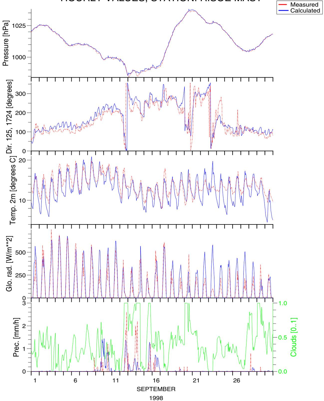
Figure 14. Comparisons of hourly values of measurements (red curves) and 12 hours forecasts using the ETA model (blue curves) for September 1998 at Risø, Denmark. Green curve is the total cloud cover from the ETA model.
