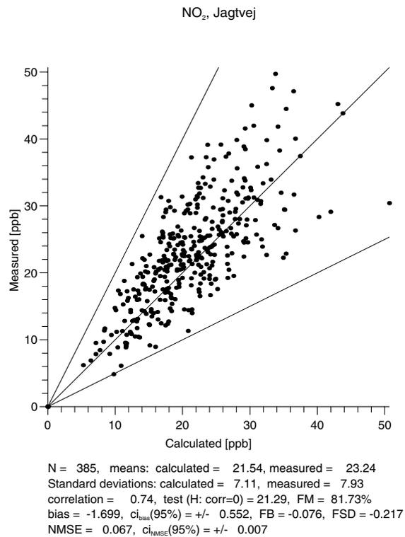
Figure 19b. Comparisons of measurements and the daily mean values of the 12 hours forecasted NO<sub>2</sub> modelled concentrations at Jagtvej, Copenhagen, Denmark for the period August 1998 to September 1999.
