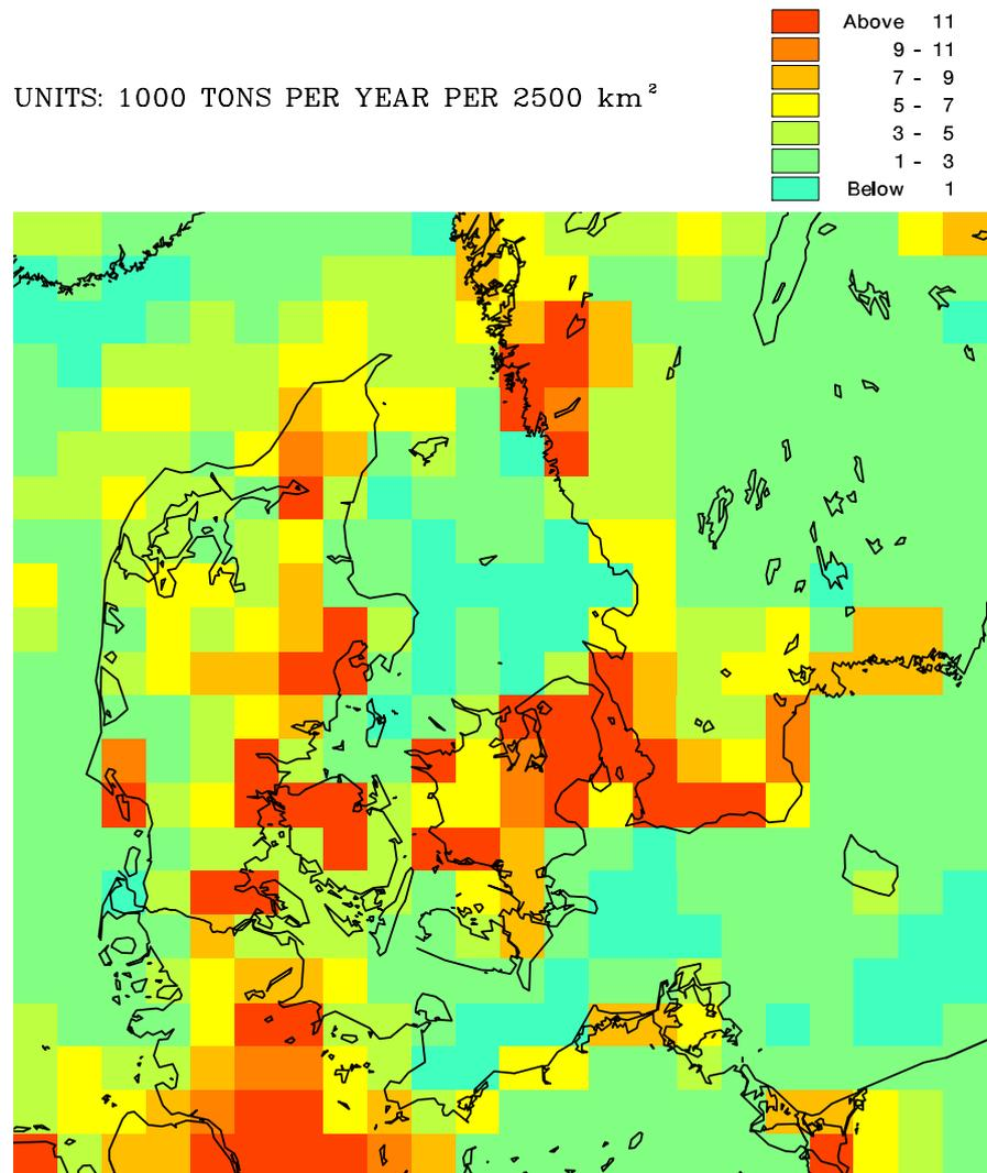
Figure 3. Example of NO<sub>x</sub> emissions used in DEOM, for Denmark. The grid resolution is 25 km x 25 km.
