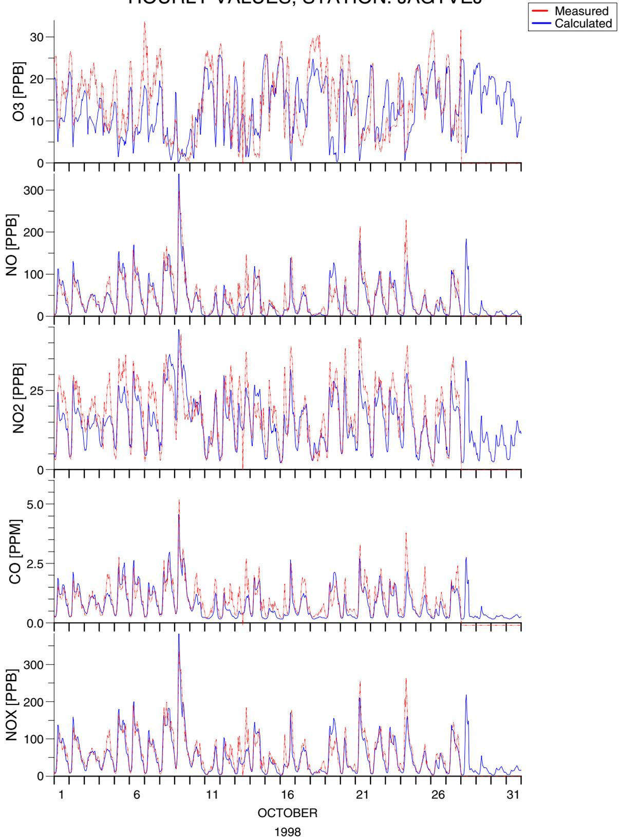
Figure 17. Comparisons of hourly values of measurements (red curves) and 12 hours forecasts using the OSPM model (blue curves) for October 1998 at Jagtvej (eastern side), Copenhagen, Denmark.
