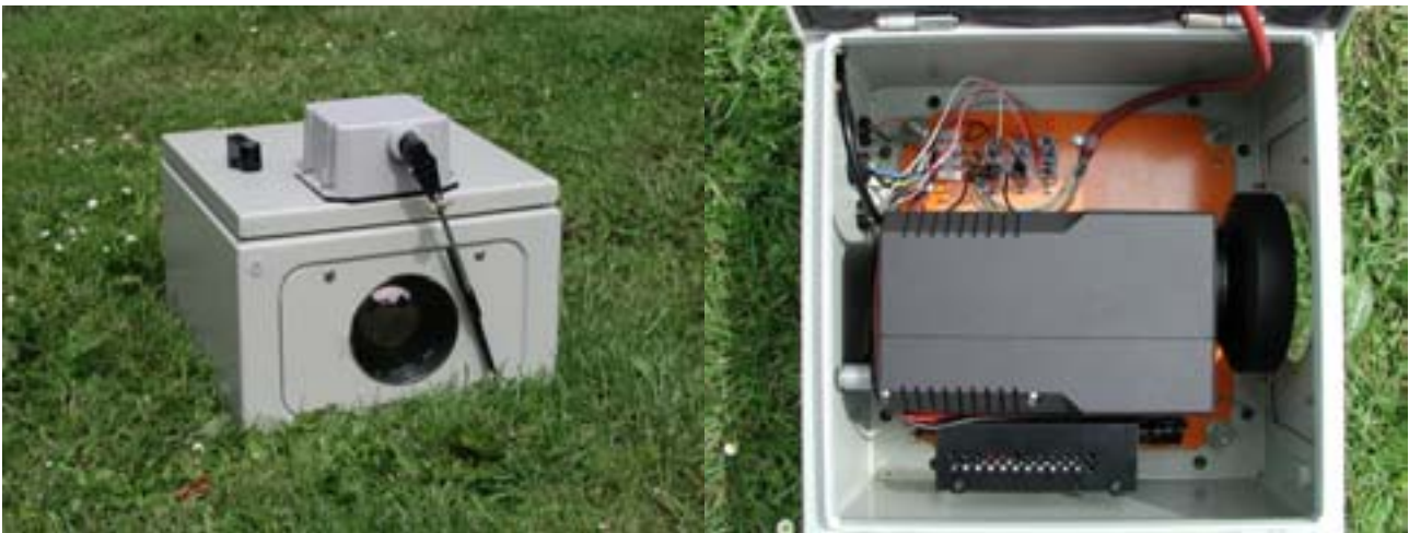
Figure 2. Waterproof metal camera housing box with windscreen wiper (left) and the thermal camera inside (right).
