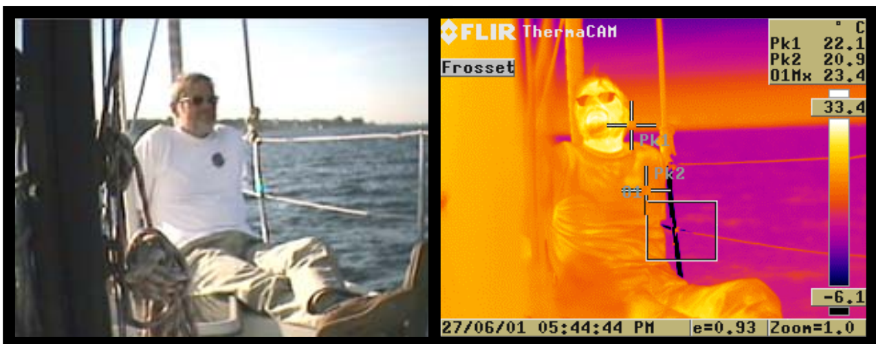
Figure 1. Photograph taken using equipment sensitive to visible light (left) and a thermogram using a heat sensitive camera (right) showing almost the same situation. The scale to the right on the thermogram shows the relationship between colours and temperatures.
