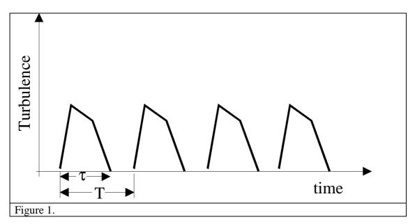
In Figure 1, T is the time period of passing vehicles and  $\tau$  is the life time of the turbulent wake created by a single vehicle.
