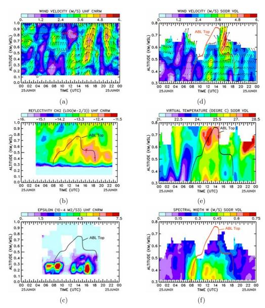
Figure 5.4: Time-height sections of UHF profiler at the Observatoire (left) and sodar-RASS at Vallon Dol (right): (a), (d) Horizontal wind velocity, (b)  $C_n^2$  reflectivity (e) virtual temperature (c) sodar Doppler spectral width, and (f) dissipation rate of turbulent kinetic energy  $\varepsilon$ . The superimposed line is the top of the atmospheric boundary layer deduced from the maximum UHF reflectivity.
