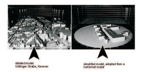
Figure 13.1: Complexity of the building structure of the real site in comparison to the building structure that was accommodated in the numerical model run
