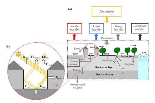
Figure 4.7: (a) Schematic representation of the SM2-U energy and water budget models with 8 surface types (pav, cova, bare, nat, roof, vega, vegn, wat, see text for explanation) and 3 soil layers, (b) Energy budget of paved surfaces.
