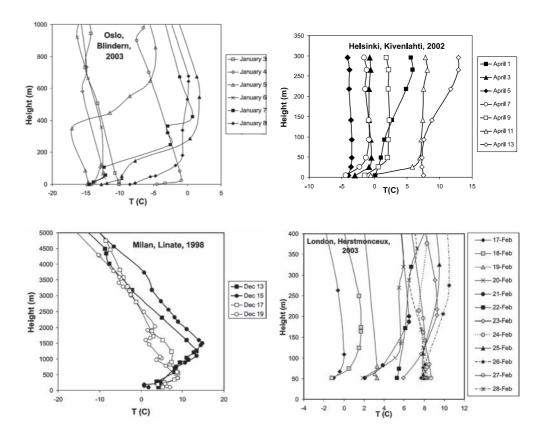
Figures 6.3. a-d: The observed temporal evolution of the vertical profiles of temperature in the four cities. For Oslo, Helsinki and London, the profiles are for midnight (00.00 UTC on the date in question), and for Milan, noon (12.00 UTC on that date). References: Sokhi et al. (2002), Kukkonen et al. (2004a,b).
