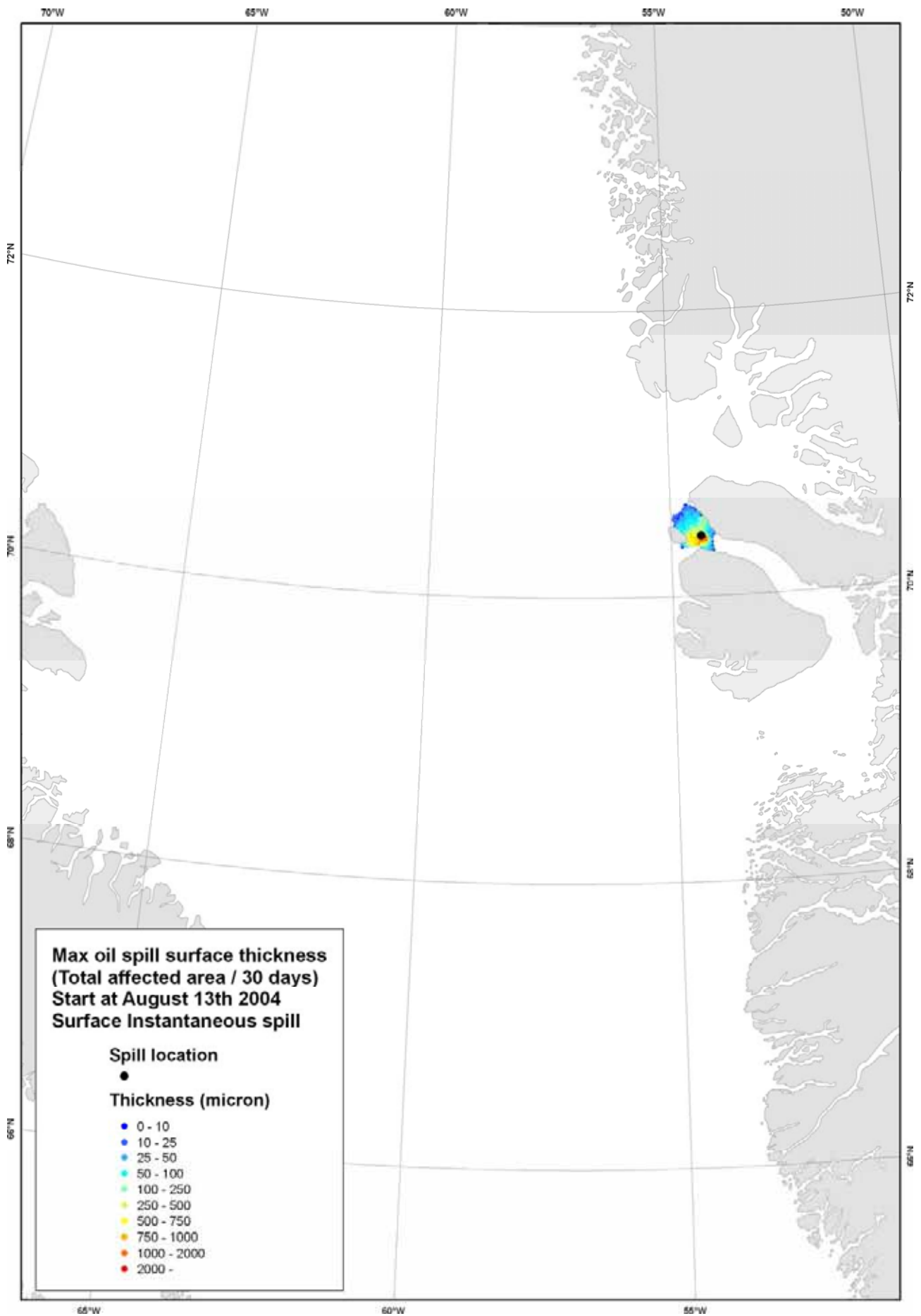
Figure A4. Maximum surface layer thickness for an instantaneous and entire area swept by an oil spill at location 6 for wind period 2 (starting on Aug. 13th 2004). From the DMI oil spill modelling report (Nielsen et al. 2006).
