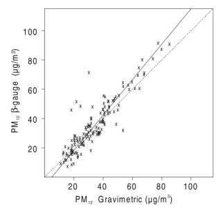
Figure 5.5 Comparison between  $\beta$ -gauge and gravimetric determination of the PM<sub>10</sub> concentration. The dotted line is 1:1 and the drawn line is the orthogonal regression line:  $y = 1.21 \text{ x} - 5.9 \text{ µg/m}^3$  ( $\rho$ =0.93).
