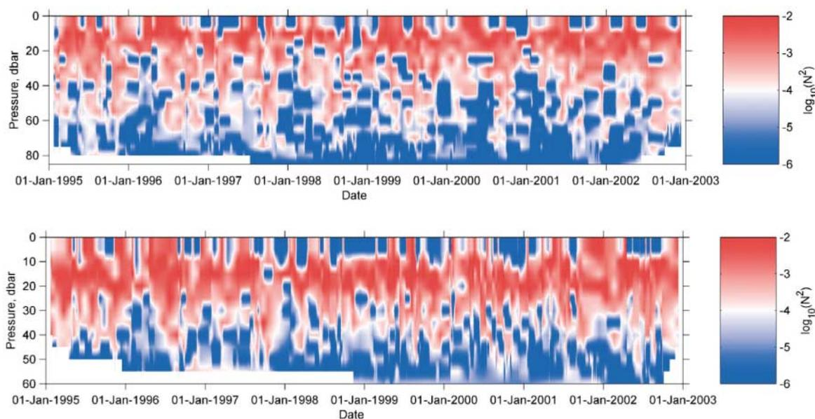
**Figure 6.4** Gridded buoyancy frequency at Fladen (upper) and Anholt East (lower). Red areas show strong stratification, while blue areas are well mixed.
