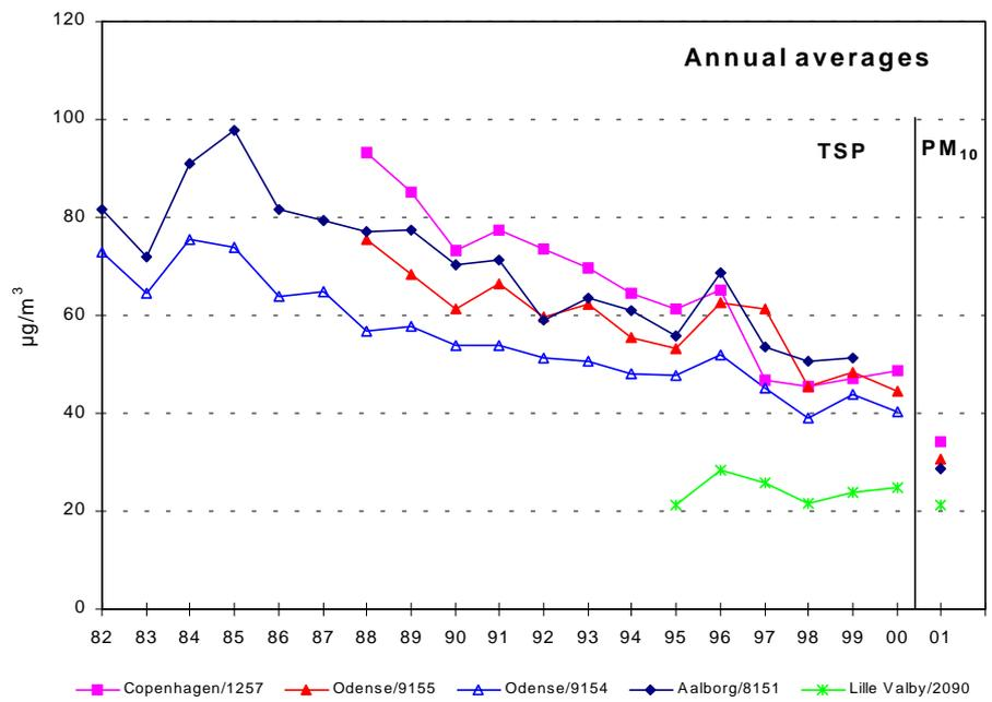
Figure 7-1 Annual averages for measurements of particulate matter
