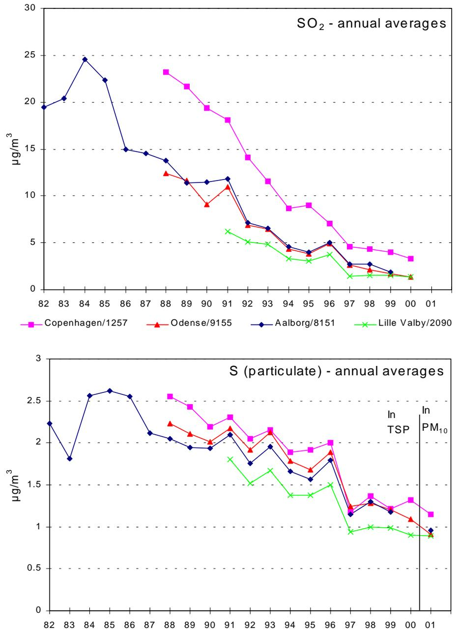
Figure 9-1 Annual averages for SO<sub>2</sub> and particulate sulphur. The results for 2000 and earlier are determined in TSP, and the 2001 results are for PM<sub>10</sub>.
