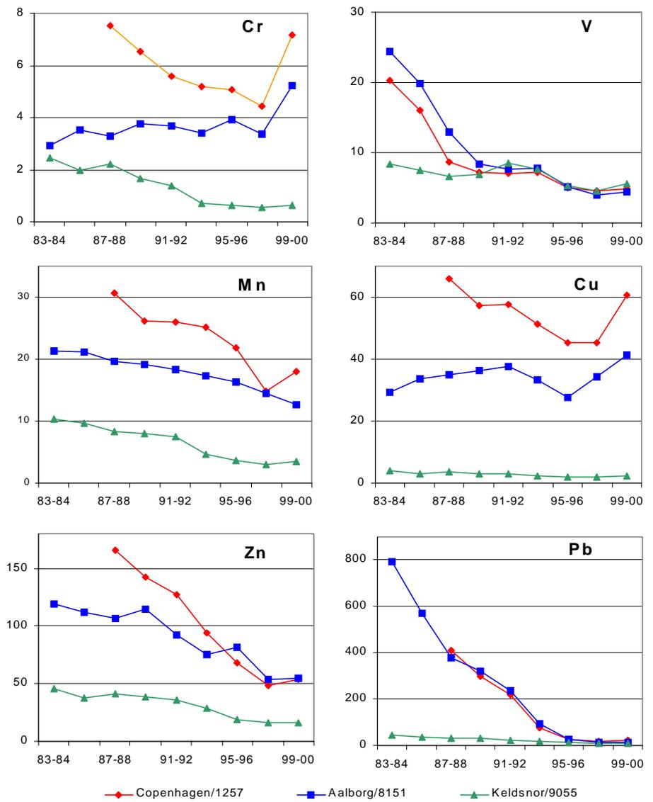
Figure 8-1 Biannual averages for Heavy Metals in particulate matter measured as TSP. y-axis units are  $\text{ng}/\text{m}^3$
