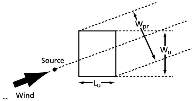
Fig. 5.3 Definition of building length, width and projected width.
