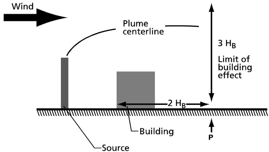
Fig. 3.3 Illustrates the criteria to determine whether the plume is affected by a building. Plume height is evaluated at the point P. If the plume height is less than  $3 H_B$ , the plume is affected by the building.
