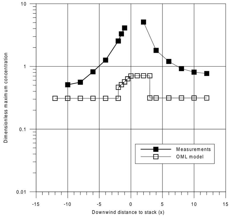
Fig. 4.2 Maximum ground-level concentration for a low stack ( $h_s/H_b = 0.5$ ), which is placed at various positions relative to the building. OML results are compared to wind tunnel measurements. The x axis indicate distance to the stack in units of building height. A cubic building is situated at the interval [0,1] along the x axis.
