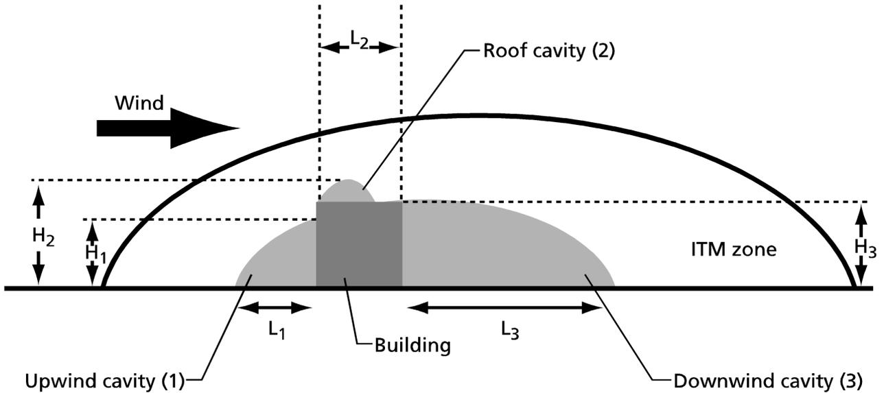
Fig. 5.1 Schematic diagram illustrating the concepts of the Genikhovich-Snyder approach: there are three cavity zones embedded in a zone of intensified turbulent mixing.
