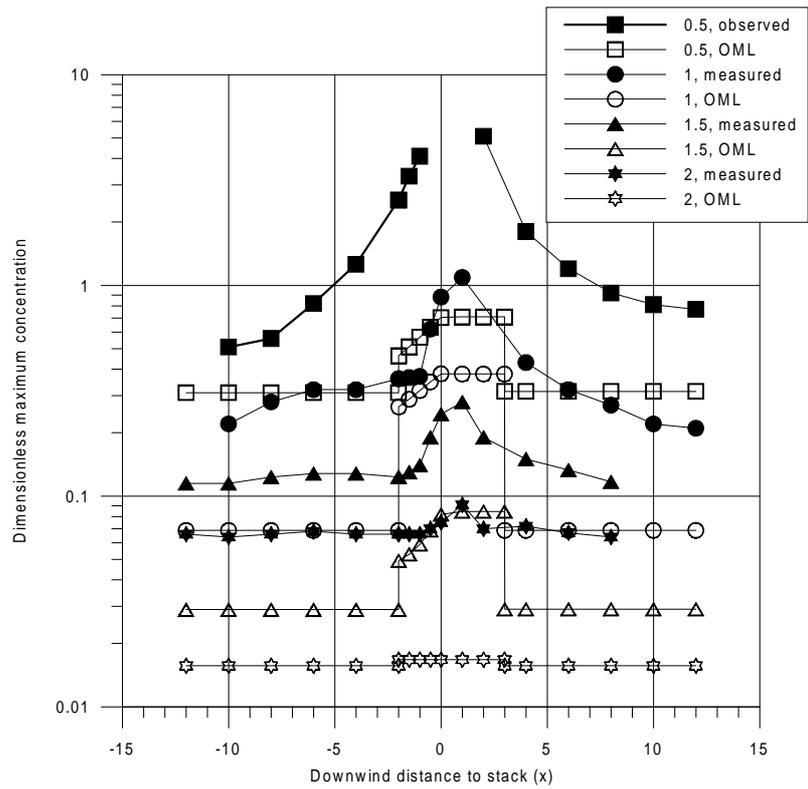
*Fig. 4.3* The curves show the maximum ground-level concentration for various stack heights (stack height in units of building height) and for various positions of the stack relative to the building. The legend indicates the value of  $h_s/H_b$  (relative stack height). A cubic building is situated at the interval  $[0,1]$  along the x axis.
