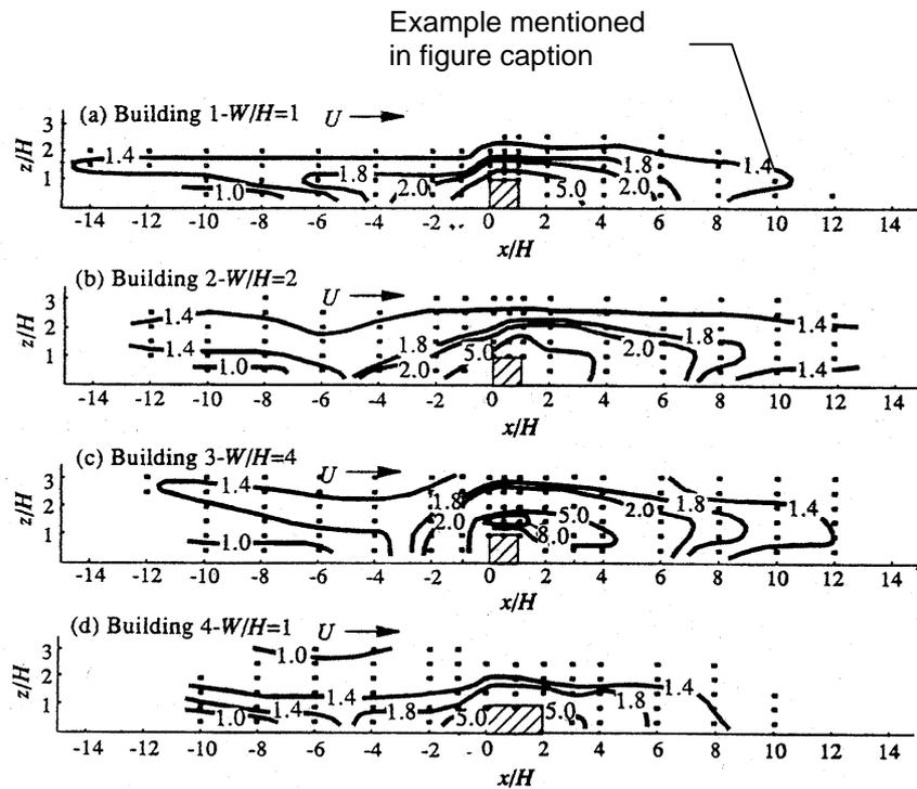
Fig. 4.1 Results from Thompson's wind tunnel investigations, where a stack was placed in various positions relative to a building. Four different building shapes were considered. Contours for BAF value for these four buildings are shown. The axes in each panel of the figure indicate the position of the stack in question.
