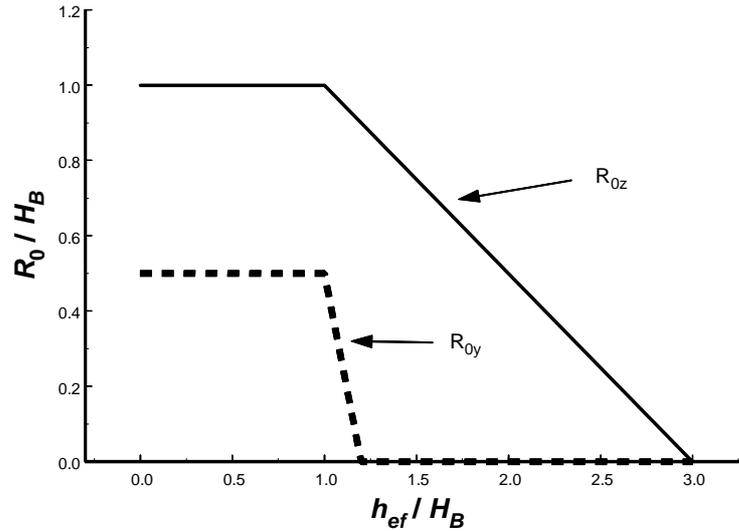
Fig. 3.1 Initial dilution radii in, respectively, vertical and horizontal direction. The radii are functions of  $h_{ef}/H_B$ .
