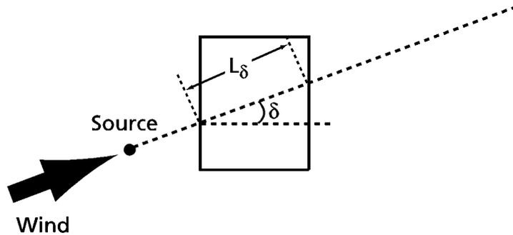
Fig. 5.4 Definition of incidence angle  $\delta$  and "traverse-building distance"  $L_\delta$ .
