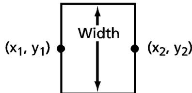
*Fig. 5.2* The co-ordinates of a rectangular building can be uniquely specified in terms of the 5 numbers indicated ( $x_1, y_1, x_2, y_2, \text{width}$ ).
