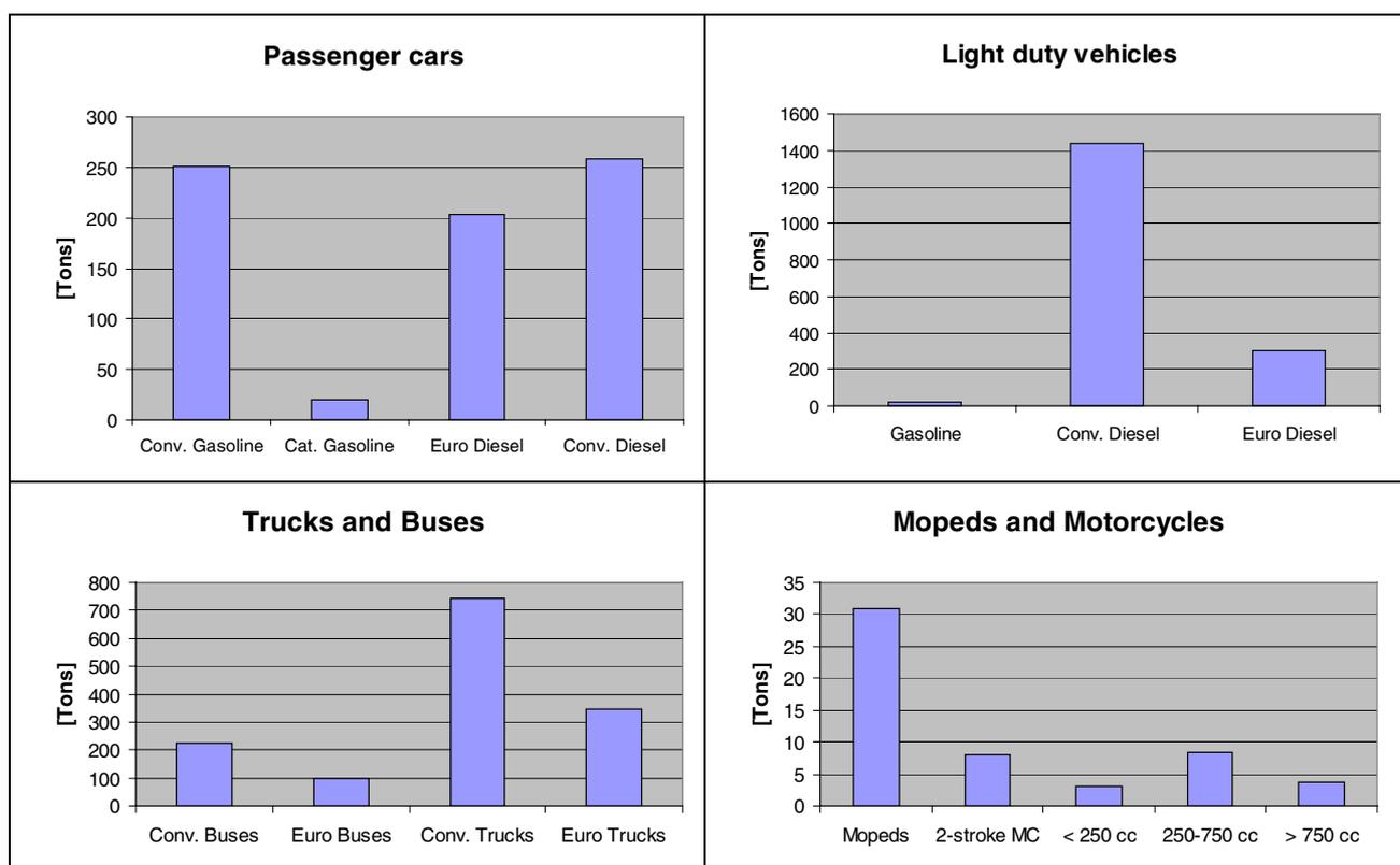
Figure 5 Each vehicle category's exhaust PM<sub>2.5</sub> emissions divided into layers
