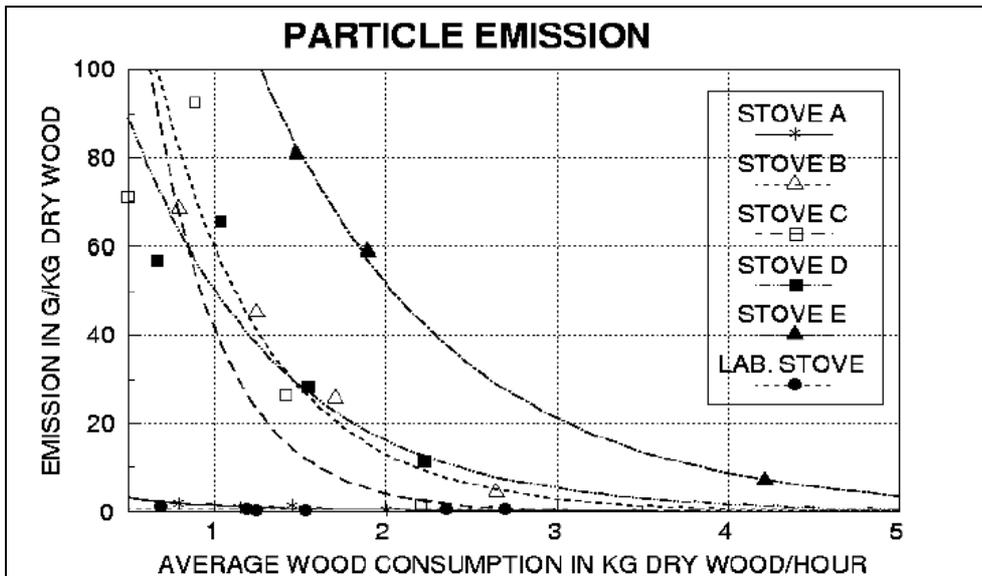
Figure A1-17 PM emission of 6 wood fired stoves. Dependency of wood consumption rate. A: Catalytic stove, B-D: old stoves, E: Open fireplace (Haakonsen and Kvingedal, 2001).
