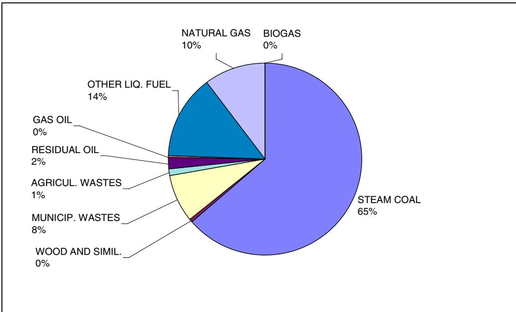
Figure A1-10 Fuel consumption of power plants > 50MW (snap 010101 and 010102)
