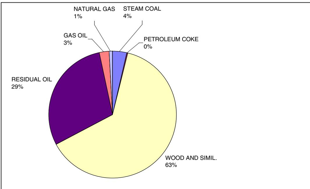
Figure A1-12 PM<sub>2.5</sub> emission from industrial boilers, gas turbines and stationary engines
