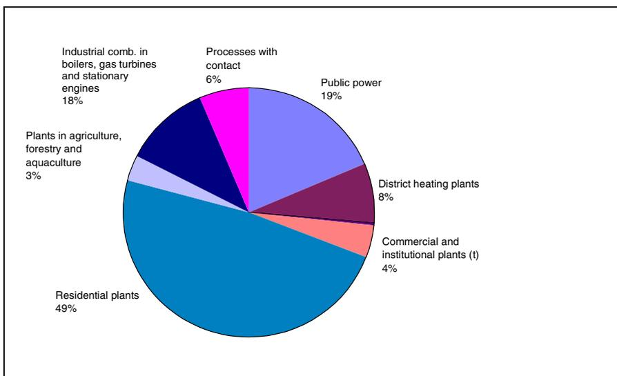
Figure A1-6 PM<sub>2.5</sub> emission of stationary combustion plants
