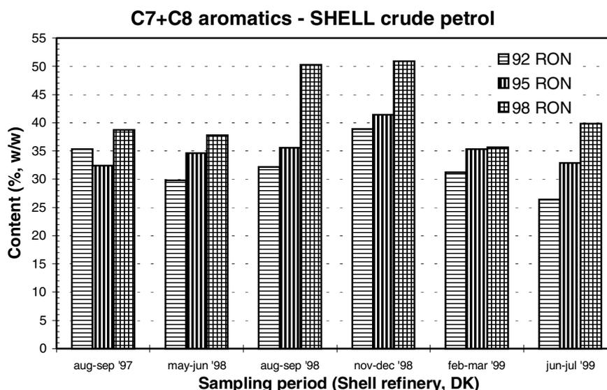
Figure 4 Average content (% w/w) of C7+C8 aromatics in crude petrol from the Shell refinery, DK, sampled and analysed in 1997-1999.
