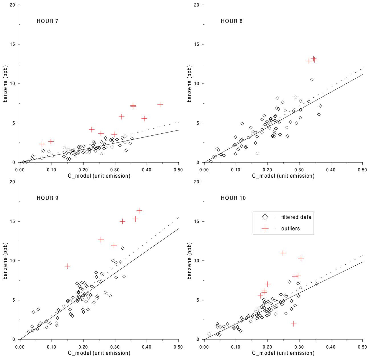
Figure 10 The procedure used for estimation of the emissions from traffic from the regression analyses is illustrated for benzene measurements in 1996 for hours 7 - 10 (ending hour). Regression lines obtained using all data are shown by dashed lines, while the regression lines for the filtered data are shown by solid lines.
