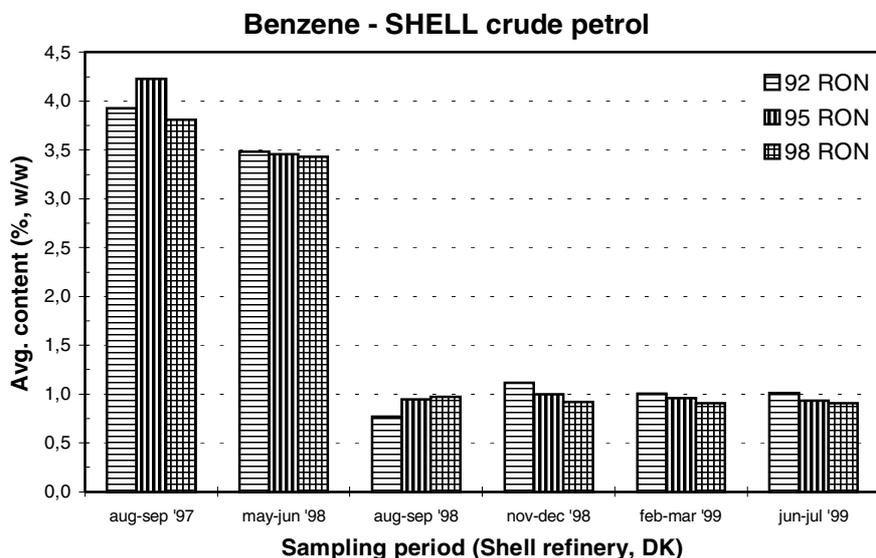
Figure 2 Average benzene content (% w/w) in crude petrol from the Shell refinery, DK, sampled and analysed in 1997-1999.
