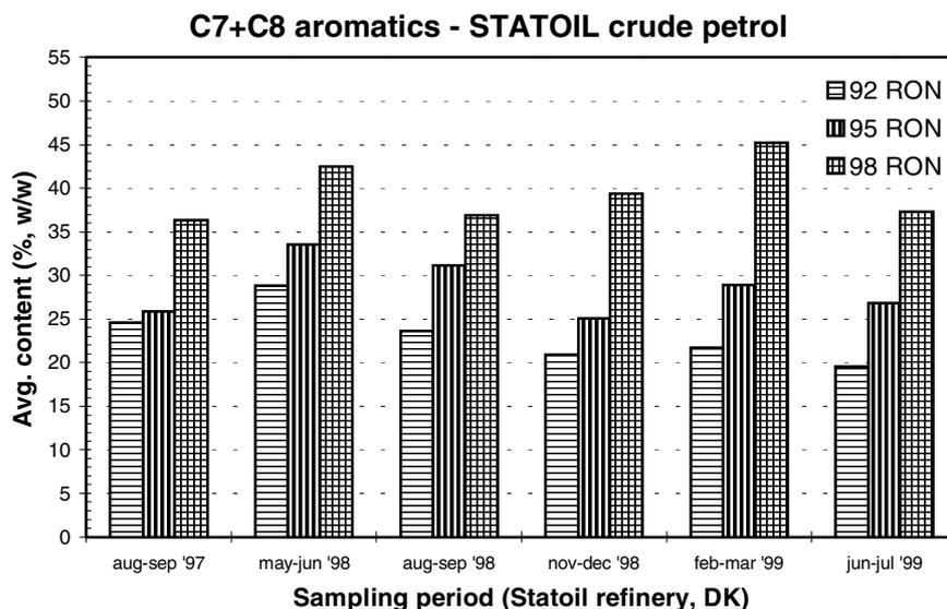
Figure 3 Average content (% w/w) of C7+C8 aromatics in crude petrol from the Statoil refinery, DK, sampled and analysed in 1997-1999.
