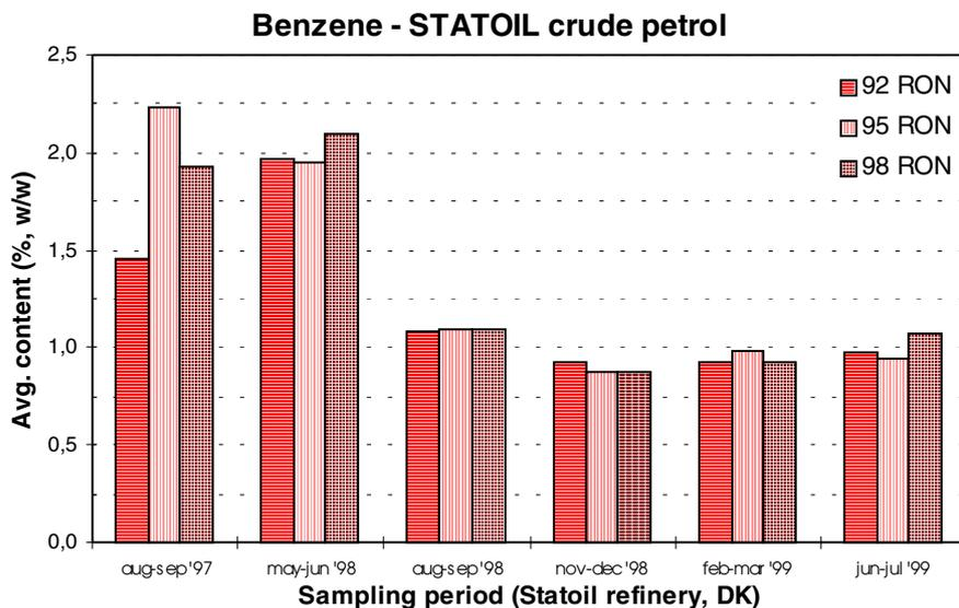
Figure 1 Average benzene content (% w/w) in crude petrol from the Statoil refinery, DK, sampled and analysed in 1997-1999.
