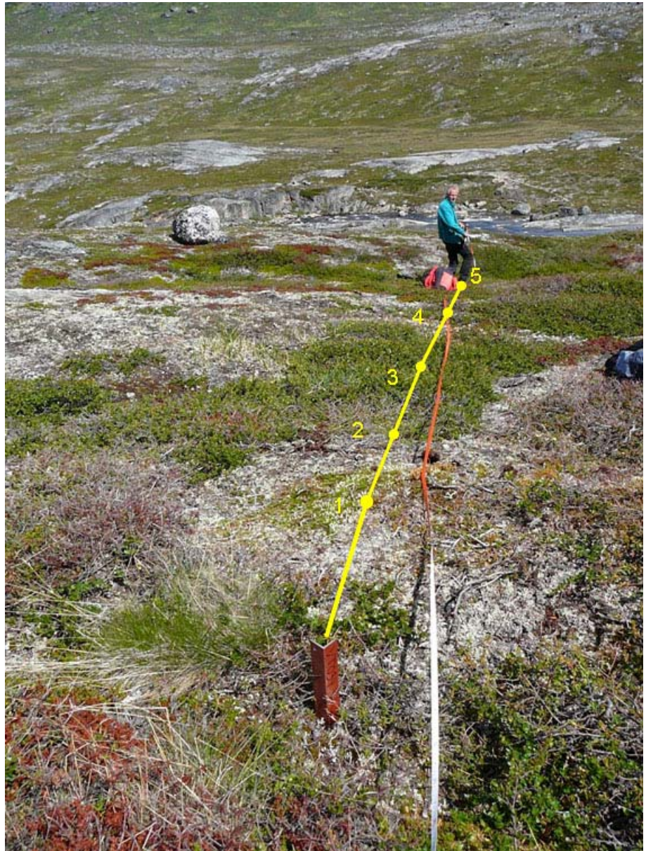
Figure 12. Location of pegs and Raunkjær circle tubes. Tubes for Raunkjær circles are shown by yellow dots and numbering is indicated by yellow numbers. Numbering starts at the peg with the lowest number and ends with tube number 10 one meter before next peg.
