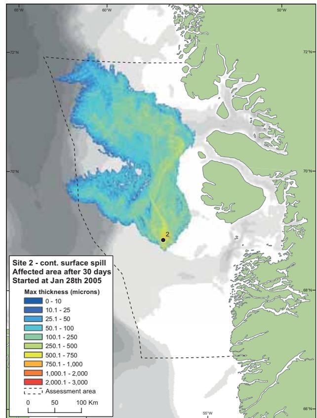
Figure 54. Examples of the DMI oil spill trajectory simulations.
