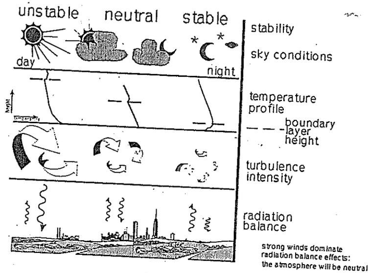
Figure 1 Qualitative presentation of atmospheric turbulence intensity, temperature profile, and the radiation during unstable, neutral and stable atmospheres.
