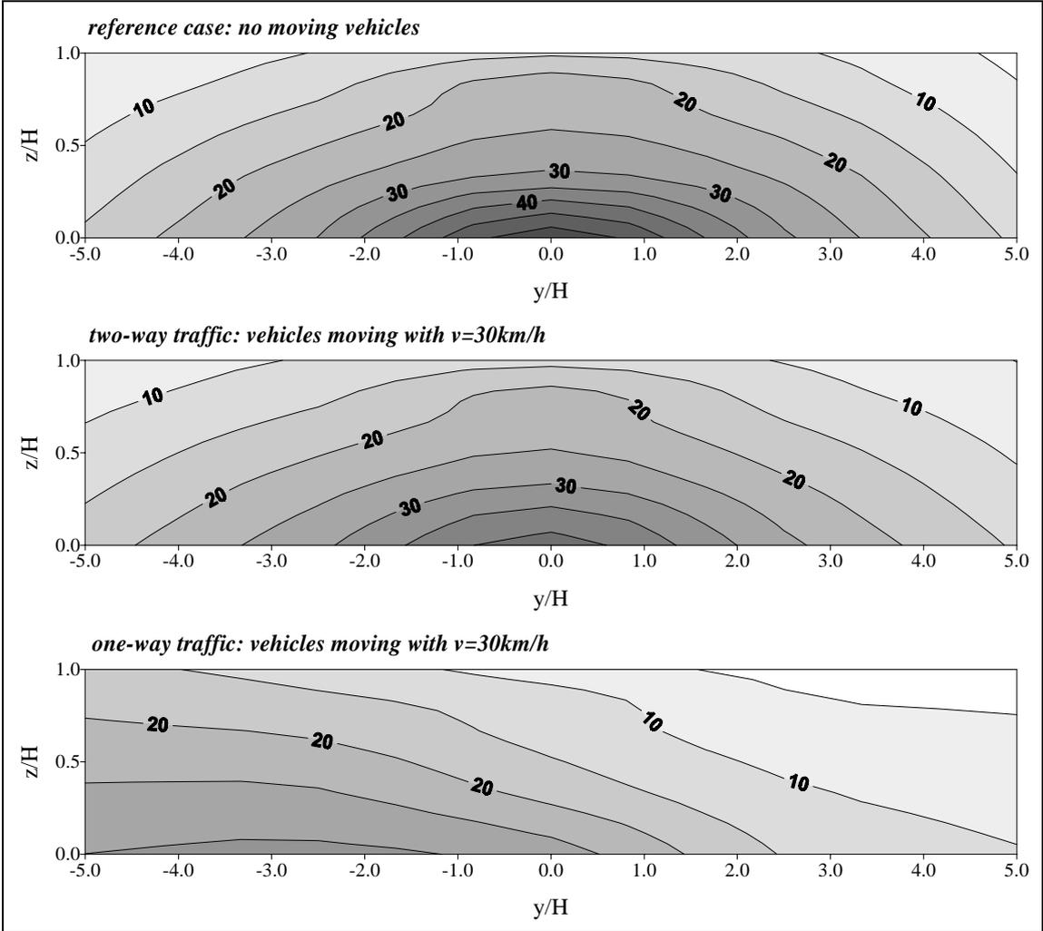
Fig. 2: Concentration patterns at the leeward canyon wall for different traffic conditions.
