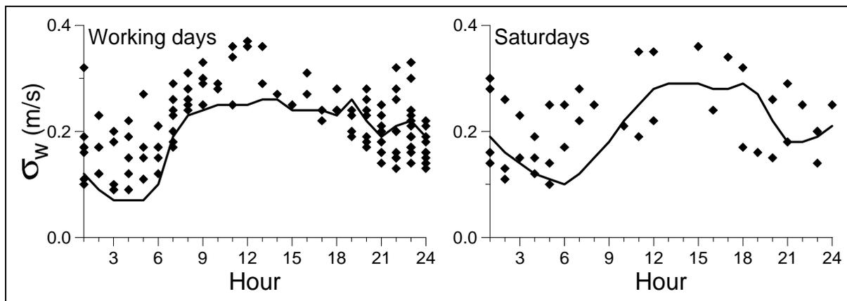
Fig. 6: Diurnal variation of  $\sigma_w$  for  $u < 1.5$  m/s on working days and Saturdays. The traffic created turbulence calculated by OSPM is shown by continuous lines.
