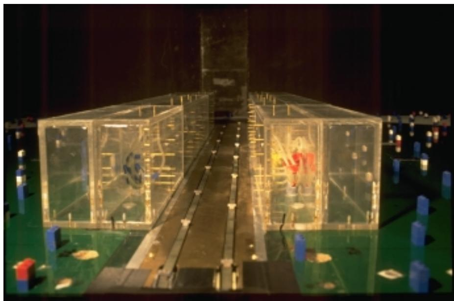
Fig. 1: Experimental set-up: street-canyon model in the wind tunnel.
