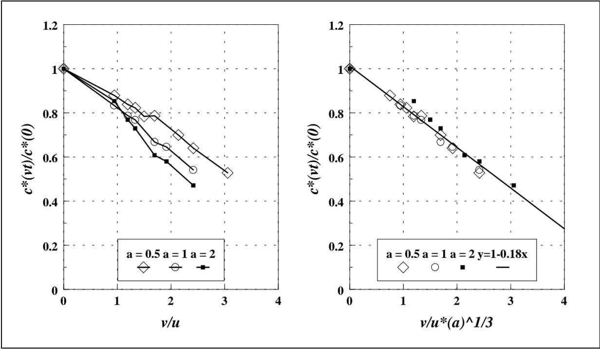
Fig. 4: Effect of moving traffic: concentration ratios at a reference point (leeward canyon wall, ground level) as function of velocity ratio  $v/u$ , with the traffic density expressed through a scaling factor  $a$ . Right side: same as left side, but with the velocity ratio  $v/u$  corrected by  $\sqrt[3]{a}$ .
