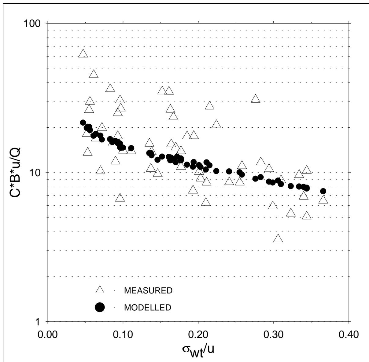
Fig. 7: Effect of traffic generated turbulence on street concentrations of  $\text{NO}_x$ .
