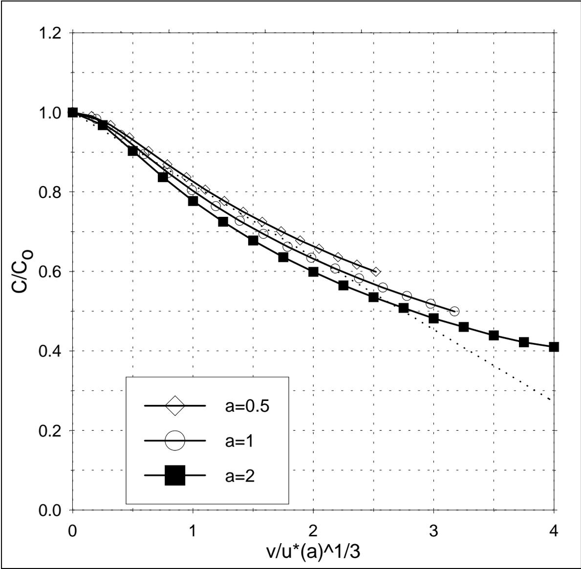
Fig. 5: Concentrations at the reference point calculated with OSPM. An approximation of the wind-tunnel data is shown by a dashed line.
