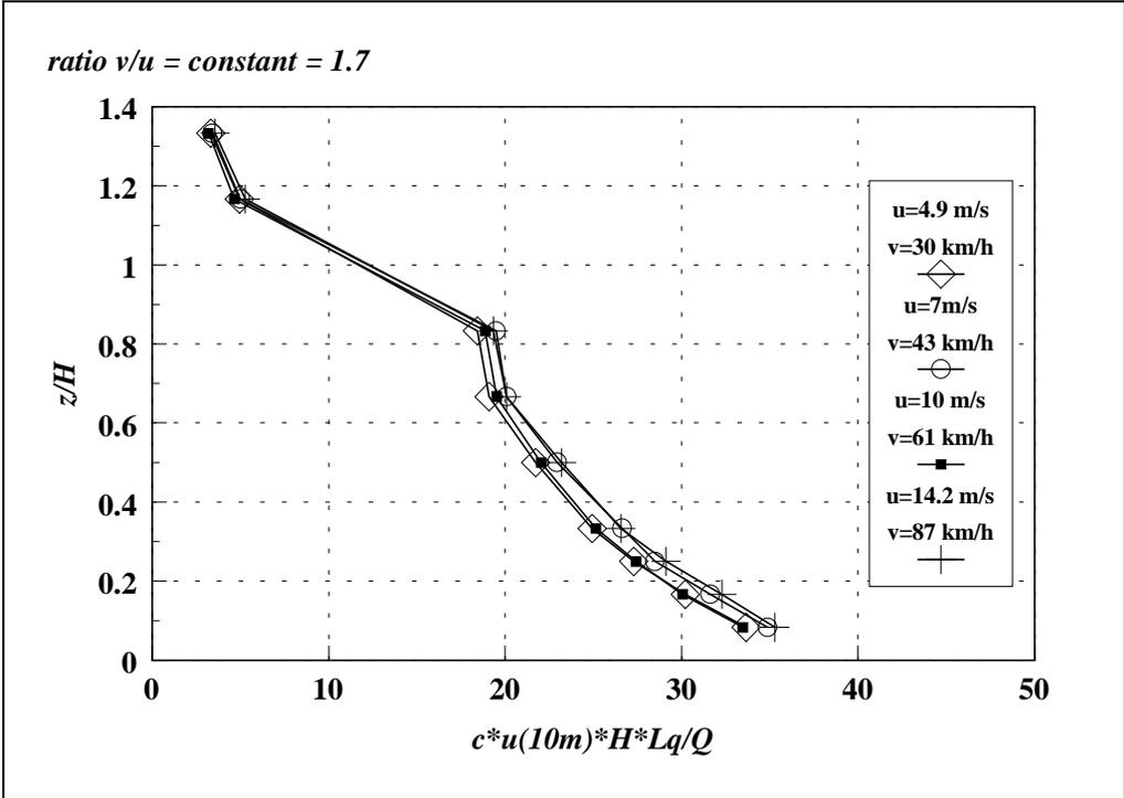
Fig. 3 Vertical concentration profiles at the leeward canyon wall (points with  $z/H > 1$  are located on the roof) for a constant ratio  $v/u = 1.7$ .
